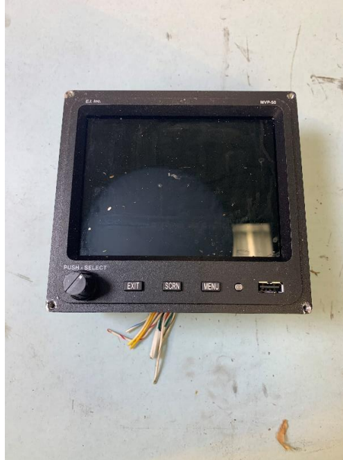
Figure 1. Condition of EI MVP-50P received by the Vehicle Recorders Division.
