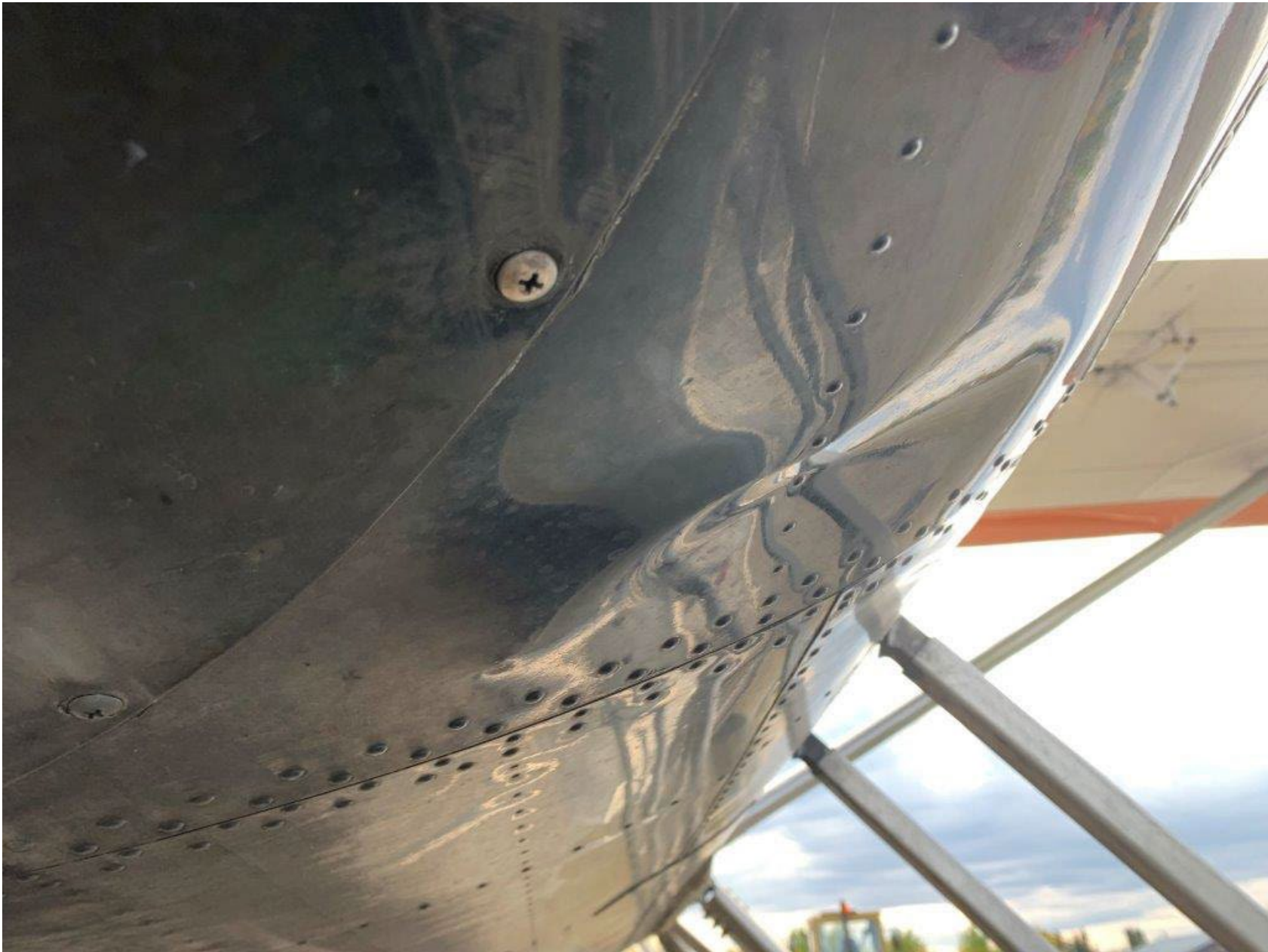
Photo 3 – View of right rear fuselage damage (Photo courtesy of Alaska Claims)
