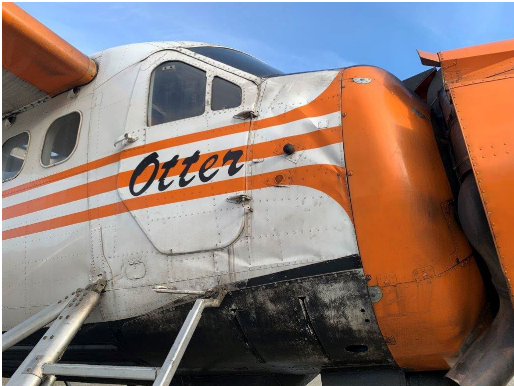
Photo 2 – View of damaged right forward fuselage (Picture courtesy of Alaska Claims)
