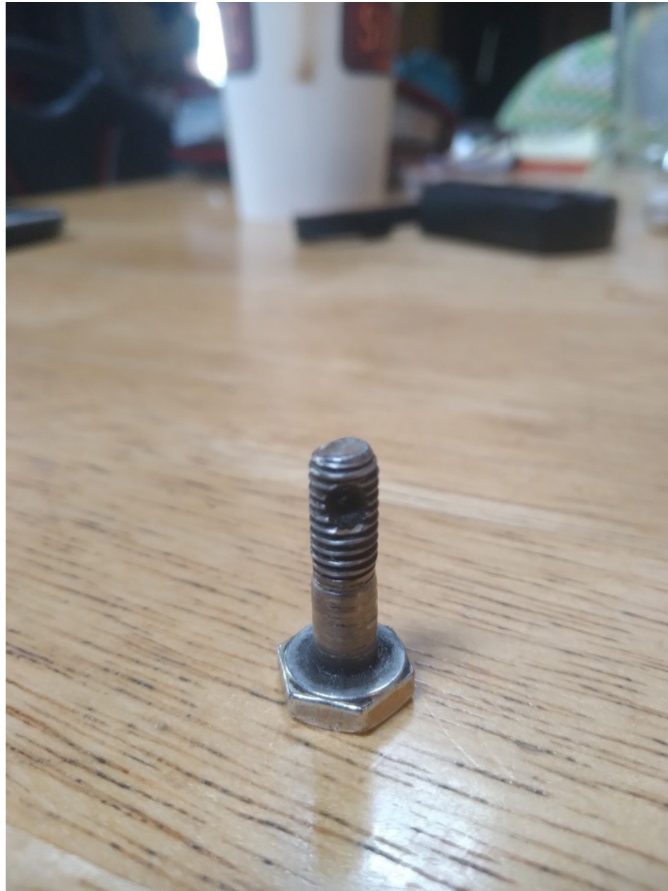
Photo 3 – View of bolt from rudder cable (Photo courtesy of the pilot)
