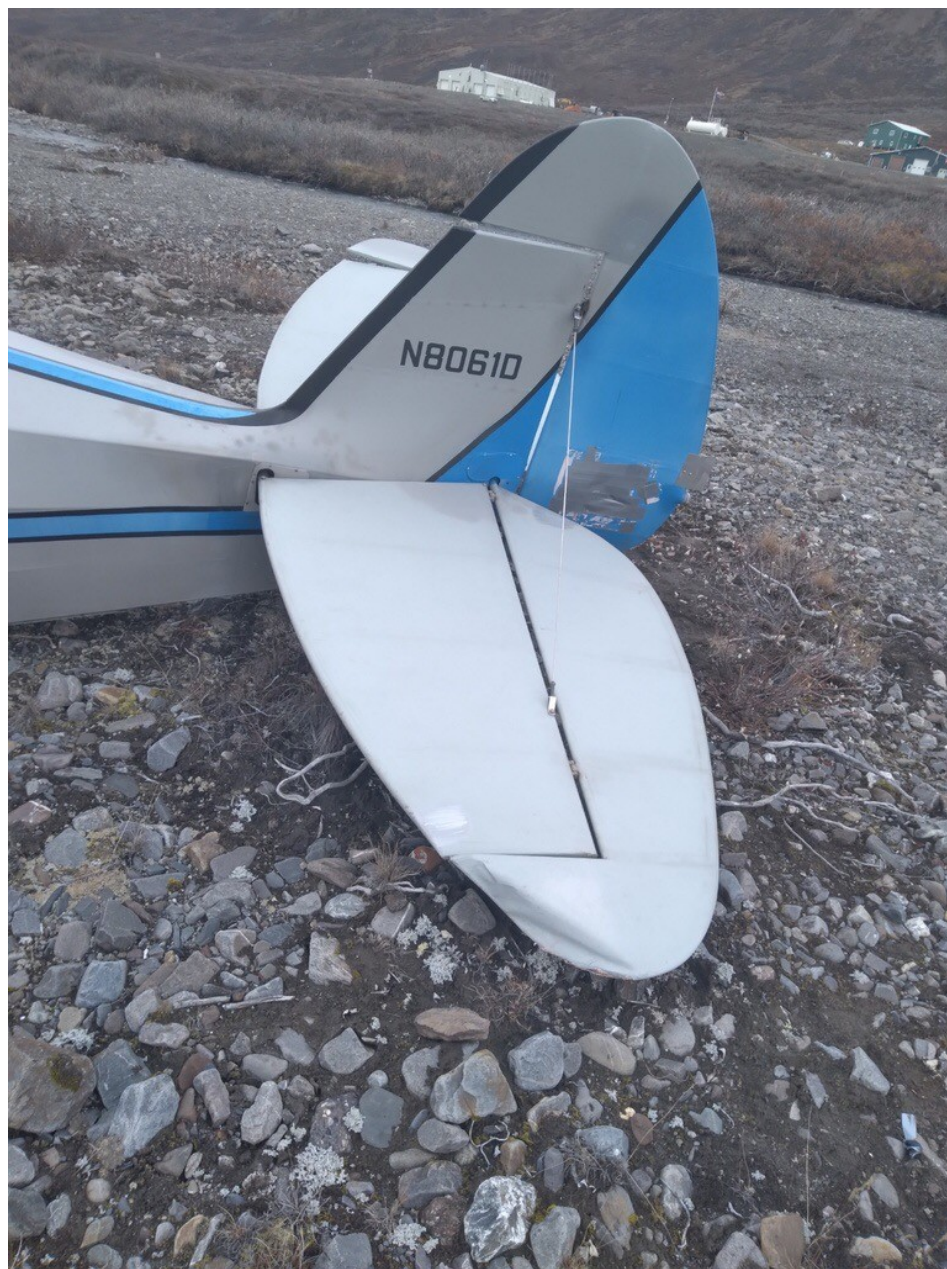
Photo 2 – View of elevator damage (Photo courtesy of the pilot)
