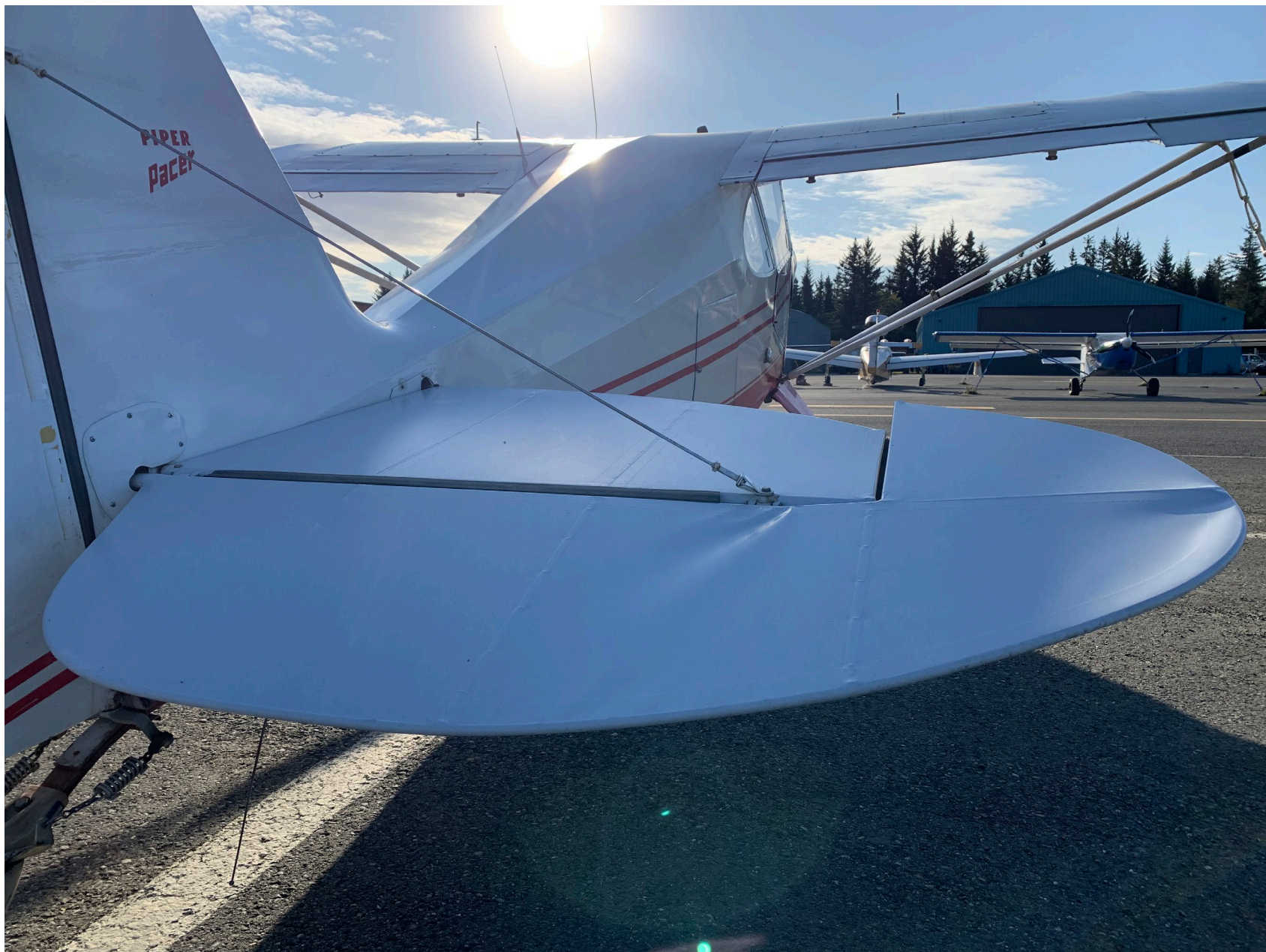
Photo 3 – Additional view of damaged elevator (Photo courtesy of the FAA)
