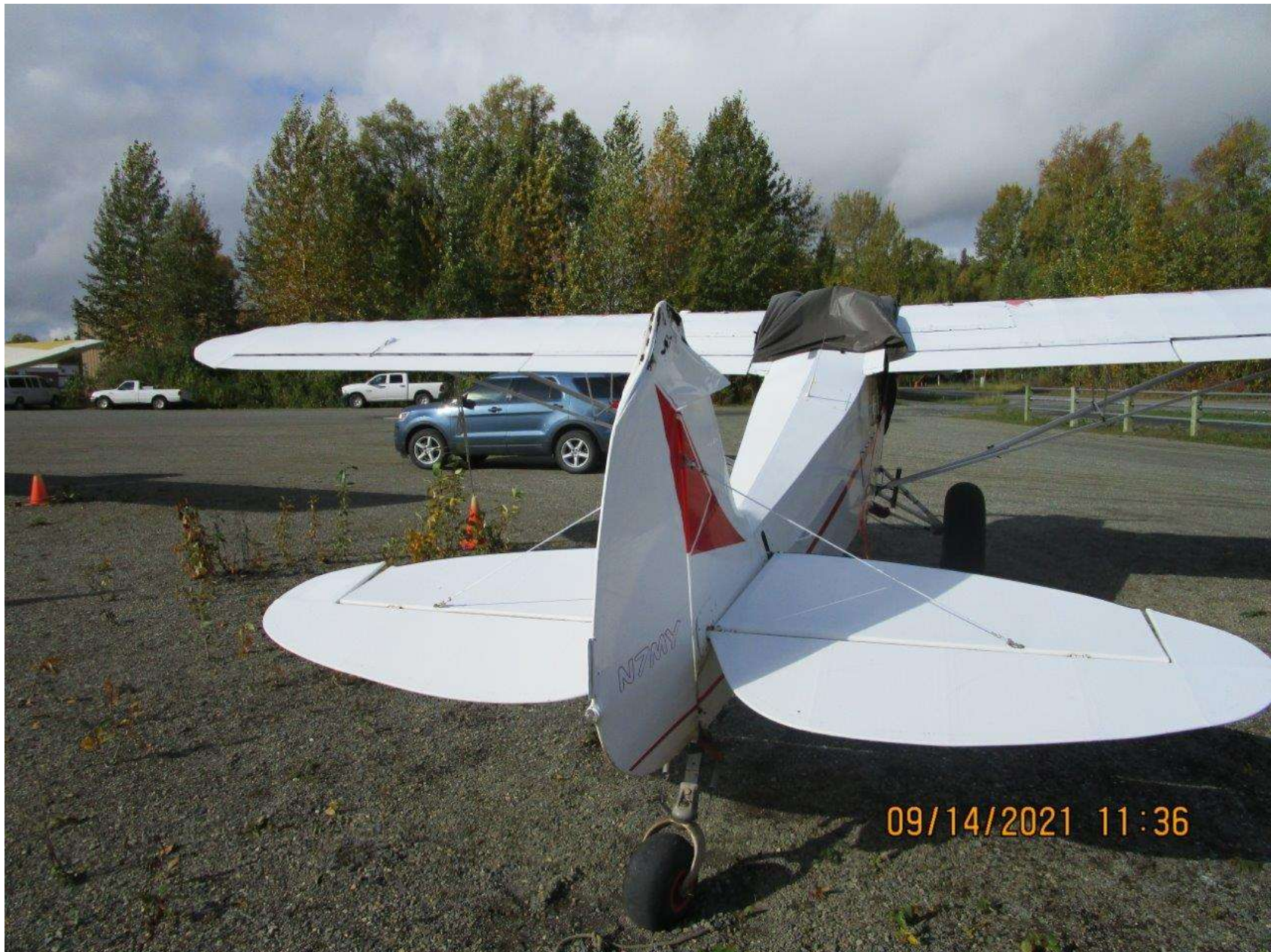
Photo 2 – Rear view of damaged empennage and left wing (Photo courtesy of the FAA)
