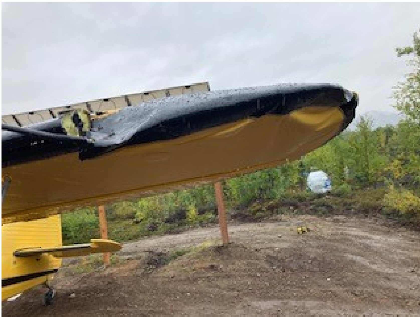
Photo 2 – Accident airplane's substantially damaged left wing. Photo provided by pilot.
