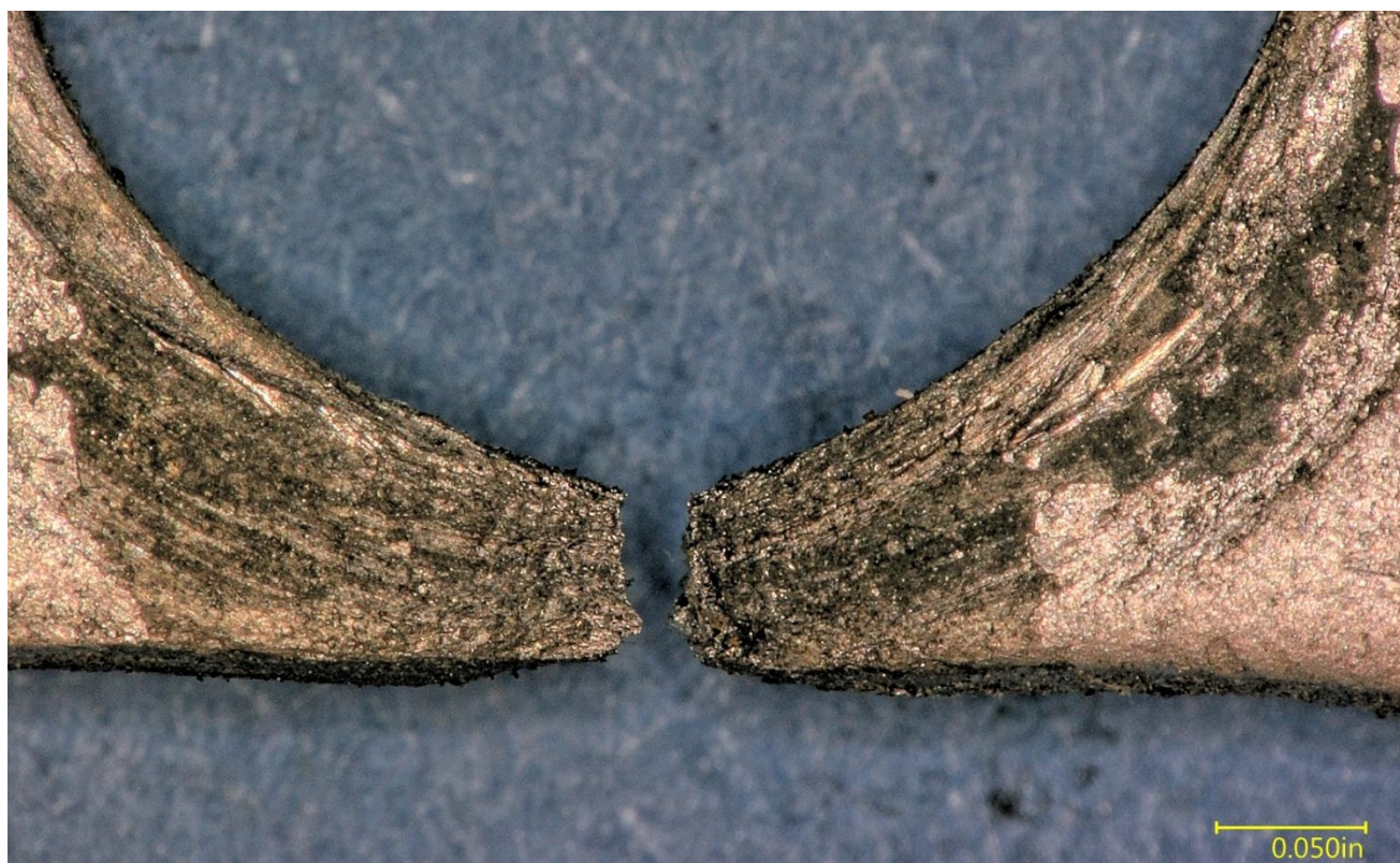
Figure 8 – View of the lower fracture around the bolt hole in the middle of Figure 2.
