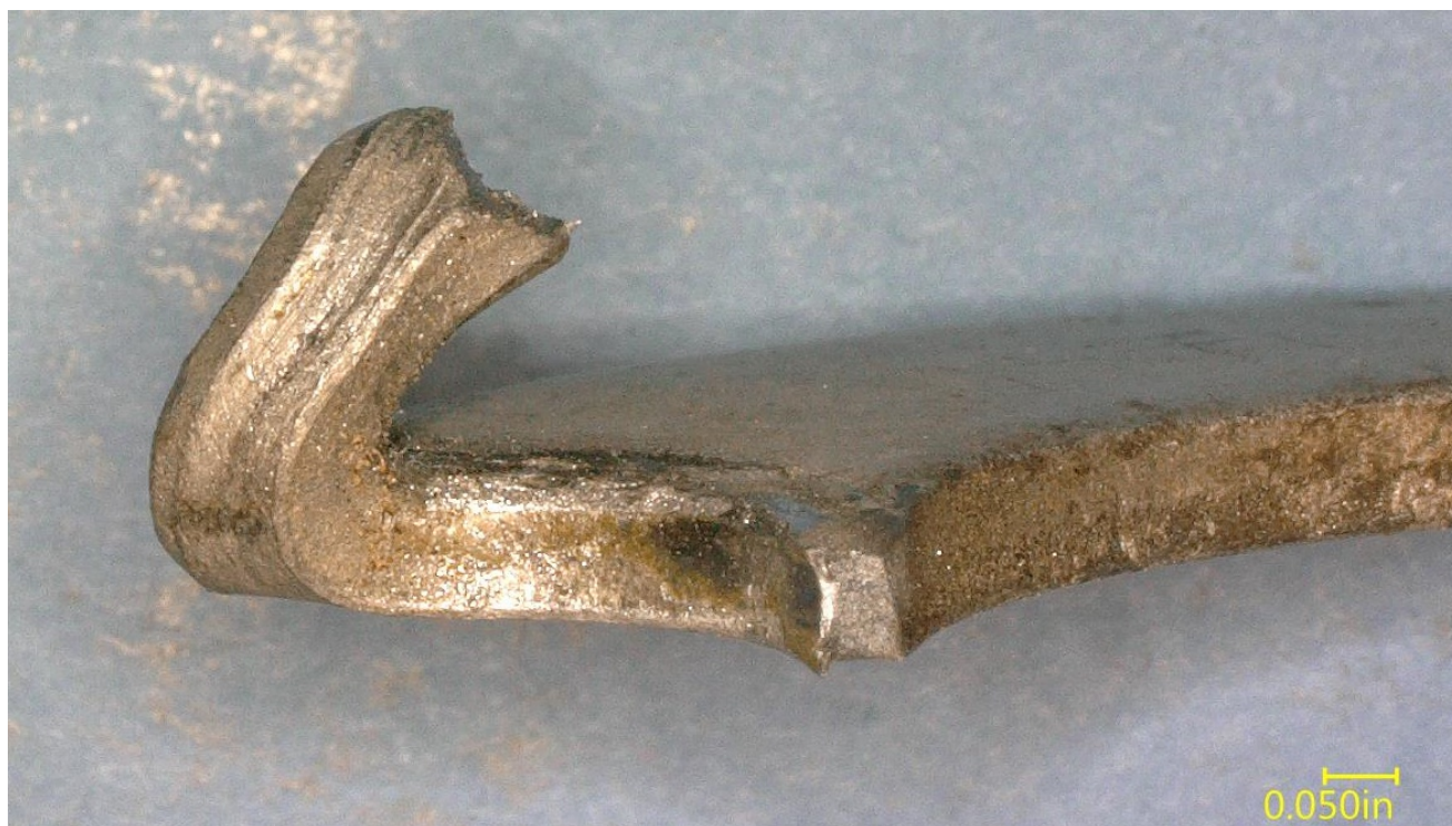
Figure 7 – View of the fracture surfaces around the bolt hole on the left side in Figure 2.
