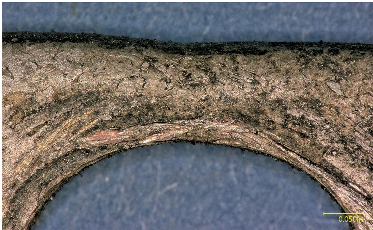
Figure 10 – The intact filament opposite the fractured one in Figure 8 and Figure 9, showing necking.
