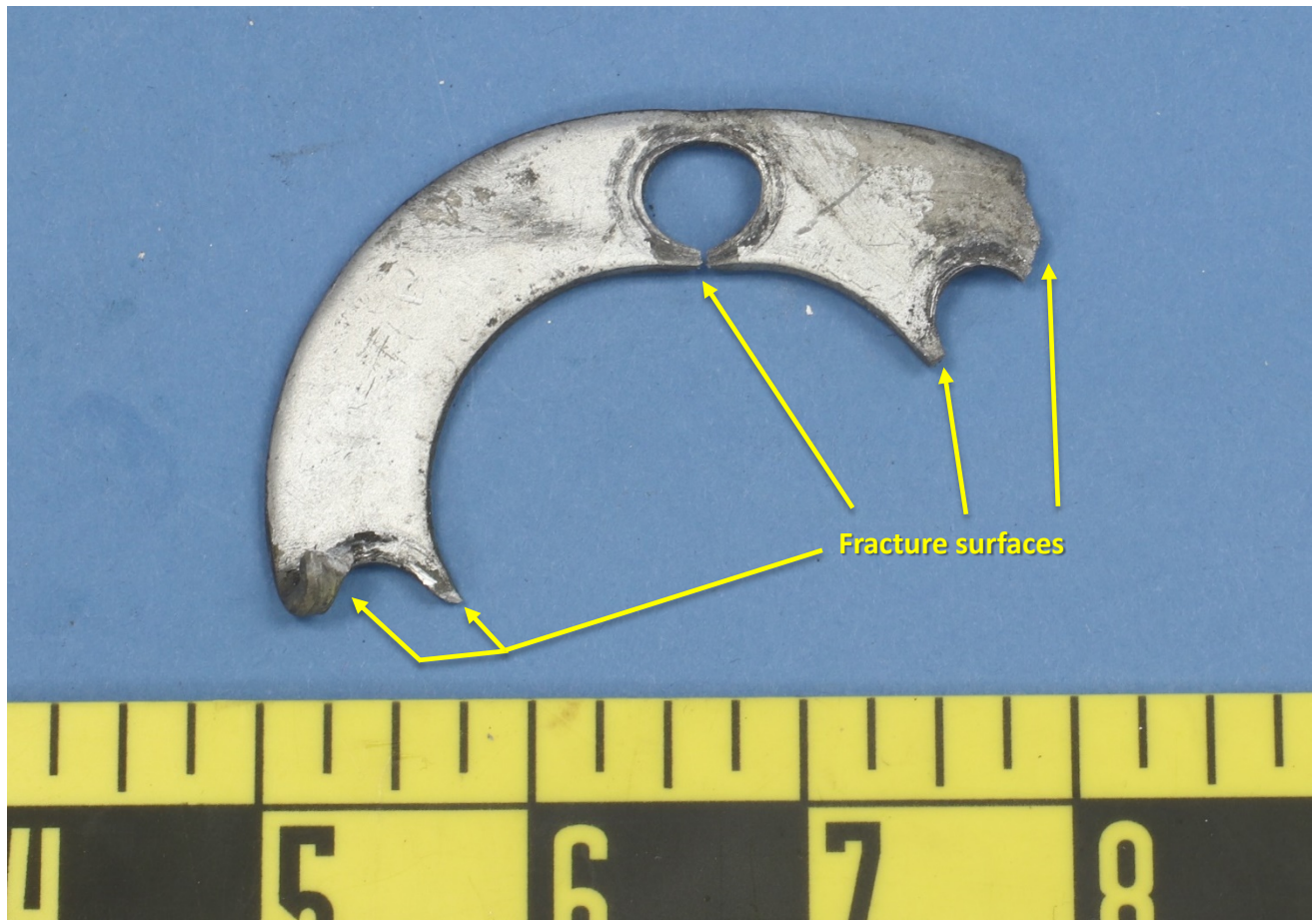
Figure 2 – View of the fractured flange remnant, showing the five fractured surfaces.
