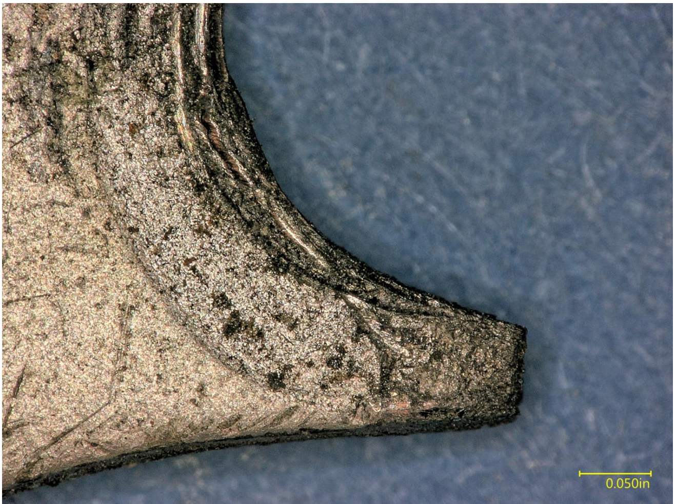
Figure 4 – Oblique view of the left fractured filament in Figure 3 near the bolt hole, showing localized thinning.
