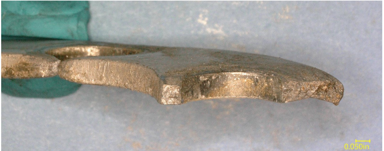
Figure 3 – View of the fracture surfaces around the bolt hole on the right side of Figure 2.
