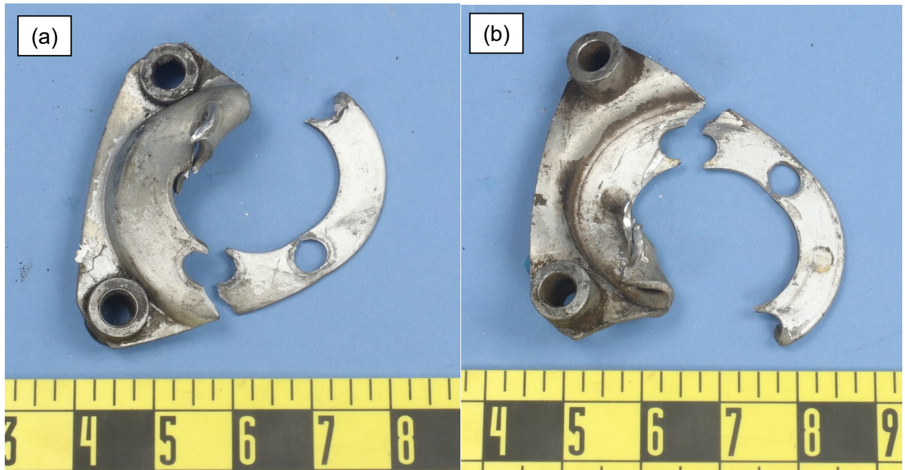
Figure 1 – View of the pieces of the torque plate from (a) the outboard and (b) inboard sides.
