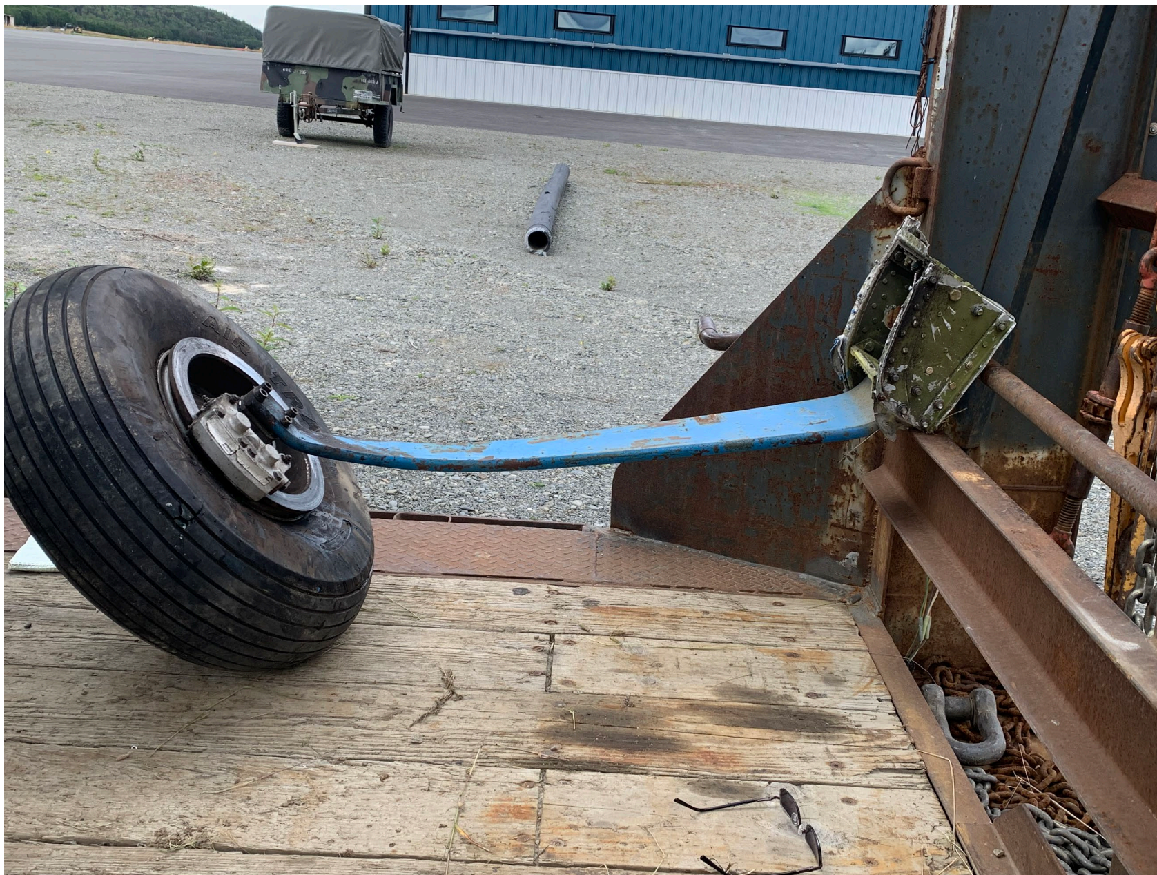
Photo 2 – Side view photo of left main landing gear “gearbox” and landing gear leg. (Photo provided by FAA)
