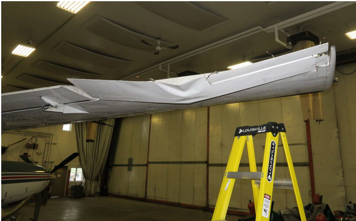
Figure 2: Damage to Right Aileron
