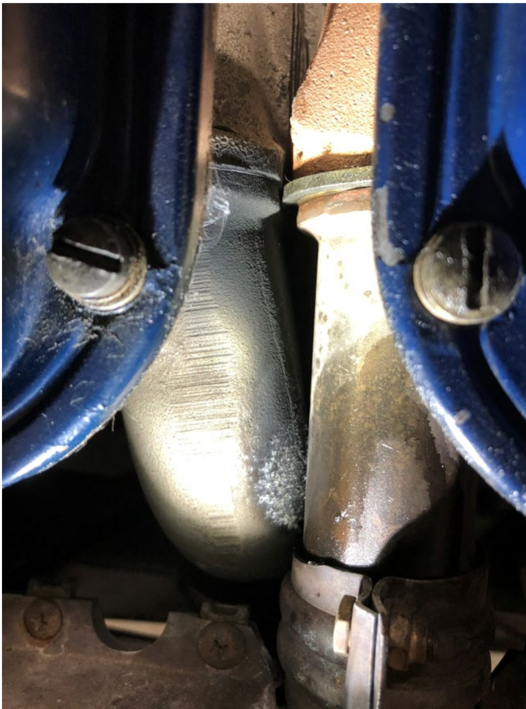
Figure 5: Exhaust from Cylinder No.2 (Right) in contact with intake tube from Cylinder No. 4 (Left)
