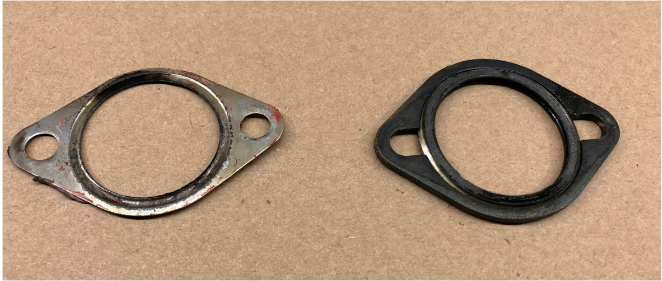
Figure 6: Stock exhaust gasket found on Cylinder No. 4 (Left): Larger exhaust gasket found on Cylinder No. 2 (Right)
