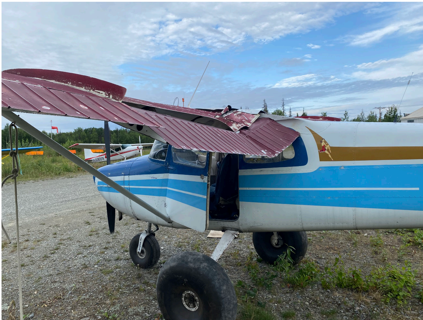
Photo 2 – Additional view of damaged left wing (Photo courtesy of the FAA)
