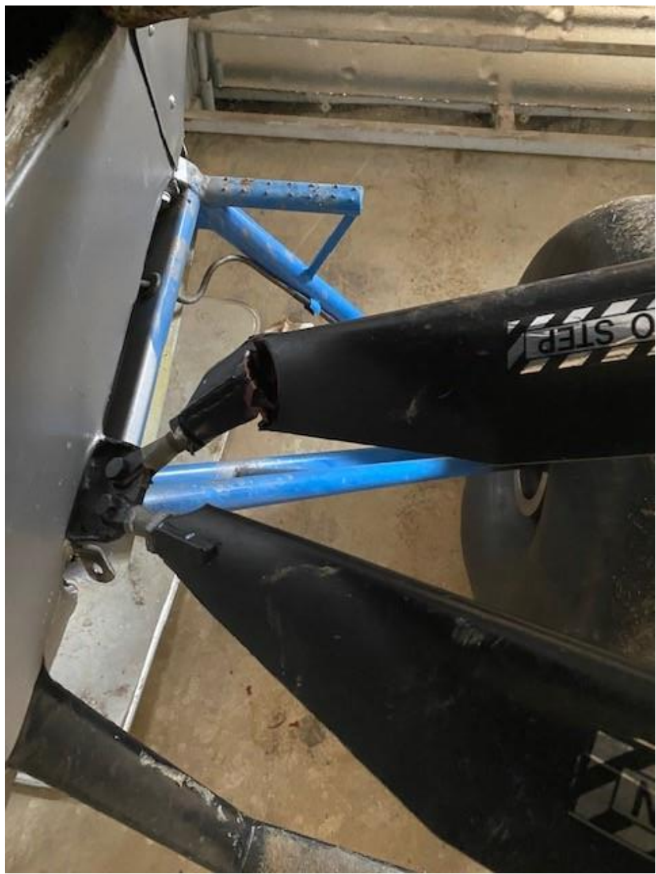
Photo 2 – View of damaged lift strut (Photo courtesy of the pilot)
