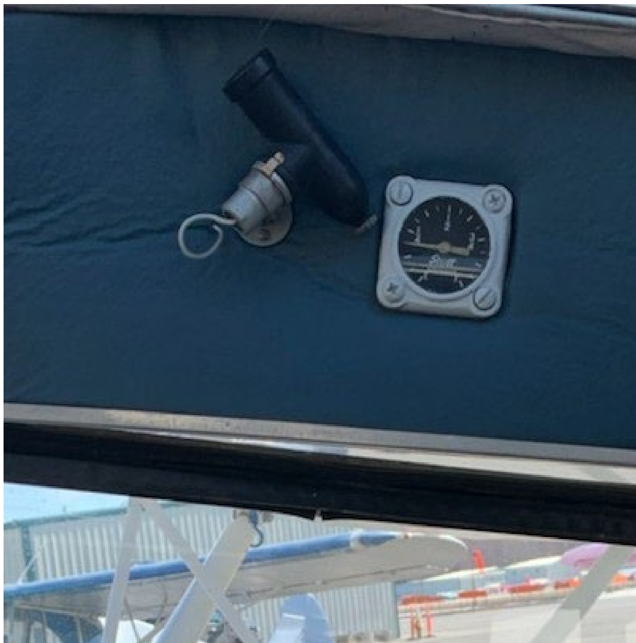
Photo 2 – Accident airplane's fuel quantity gauge. Photo provided by That Old Shop.
