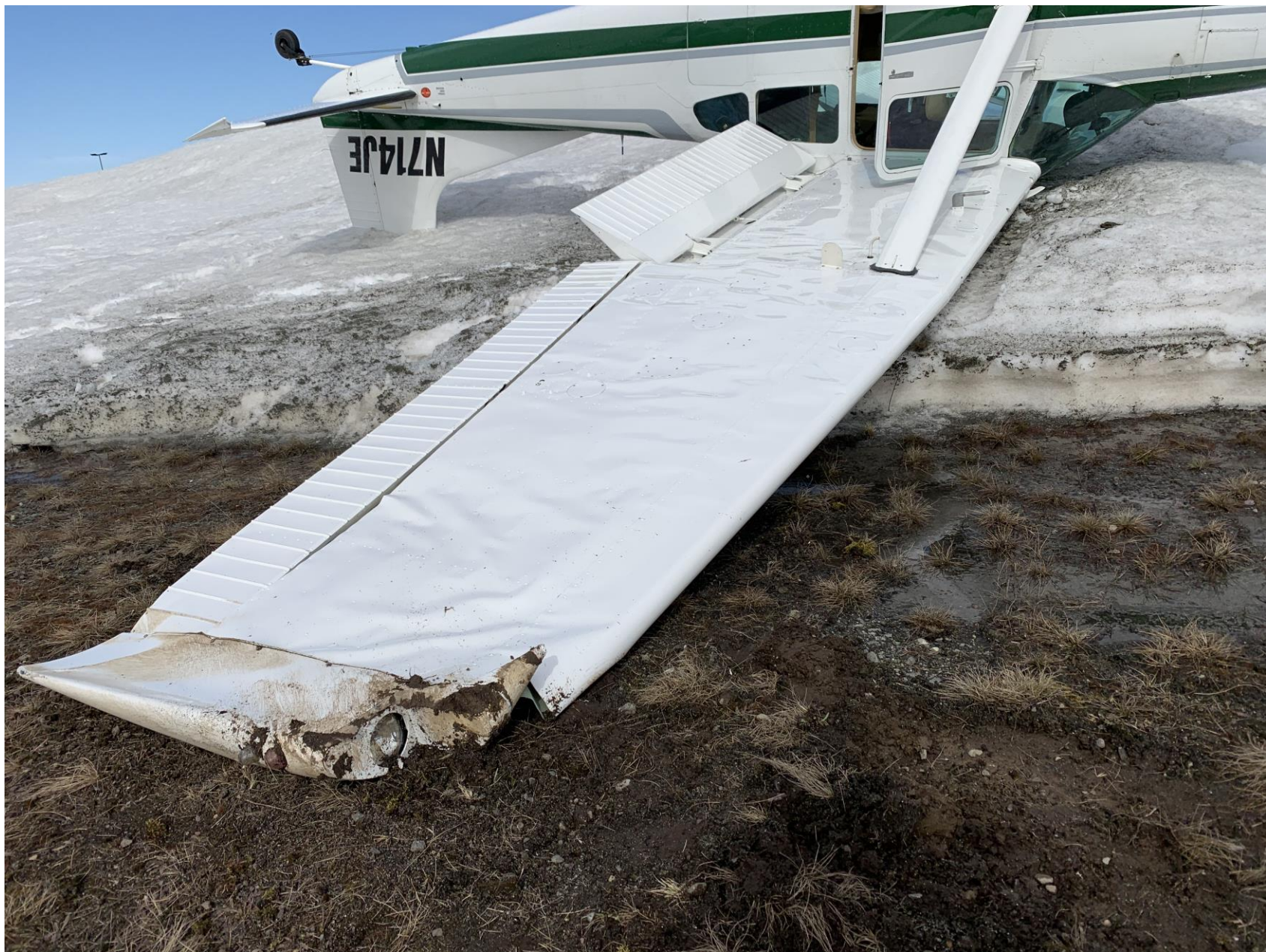
Photo 1 – View of damaged wing (Photo courtesy of Airport Operations)
