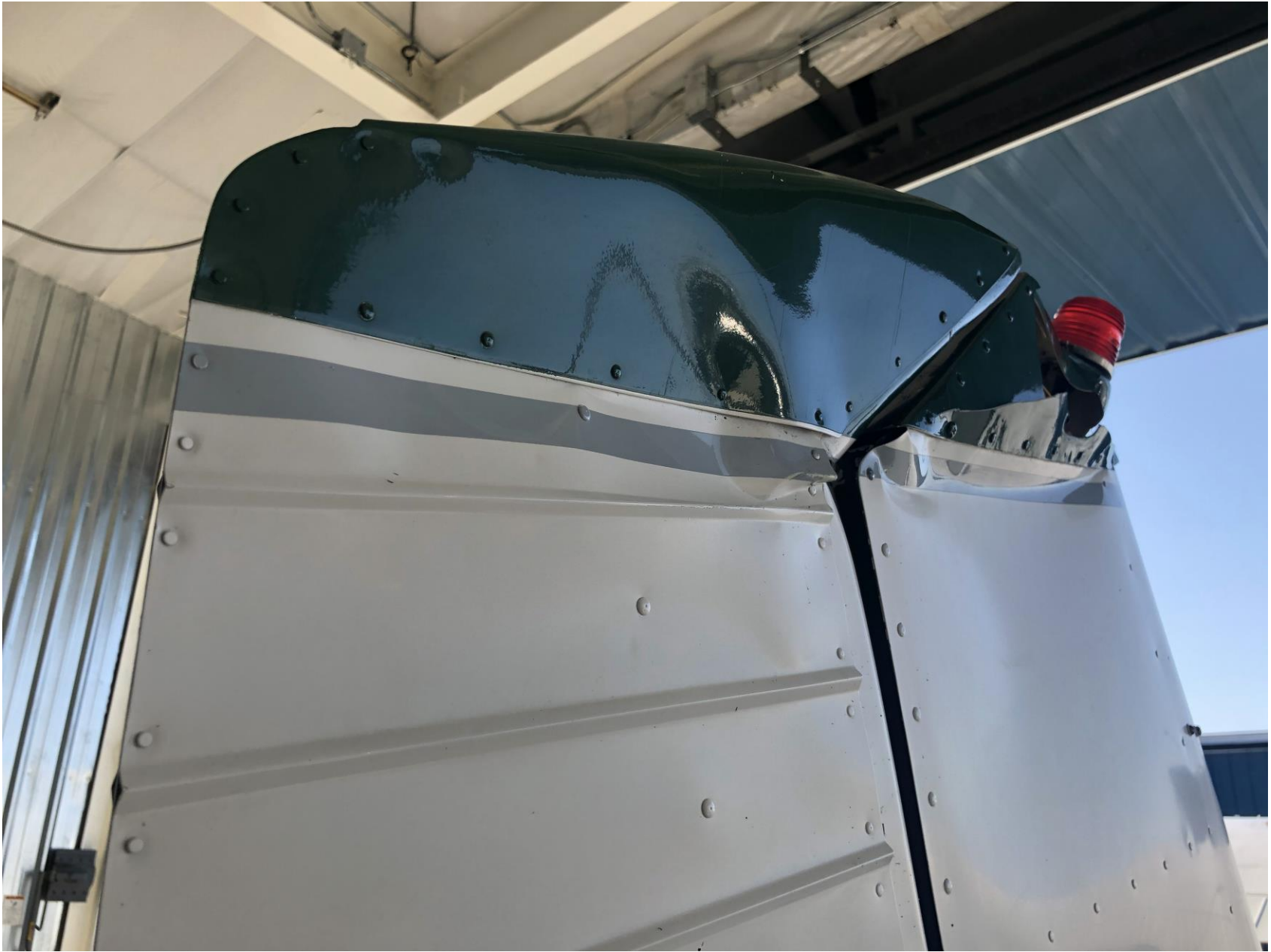
Photo 2 – View of damaged rudder (Photo courtesy of Alaska Claims Services, Inc.)
