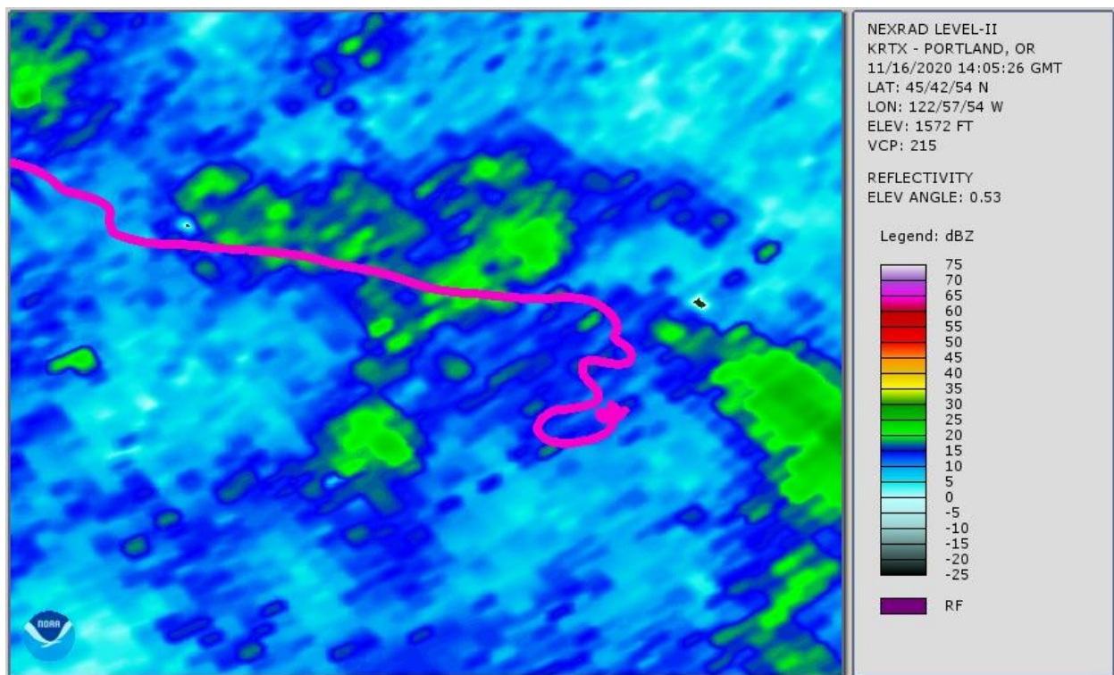
Figure 12 - NWS KRTX WSR-88D 0.53° base reflectivity scan for 0605 PST with flight track
