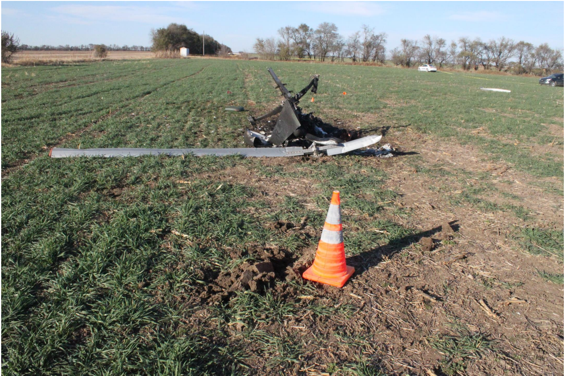
Photo 1 – Picture of accident gyroplane, the cone indicates a mark where the rotor struck the ground (Photo courtesy of the FAA)
