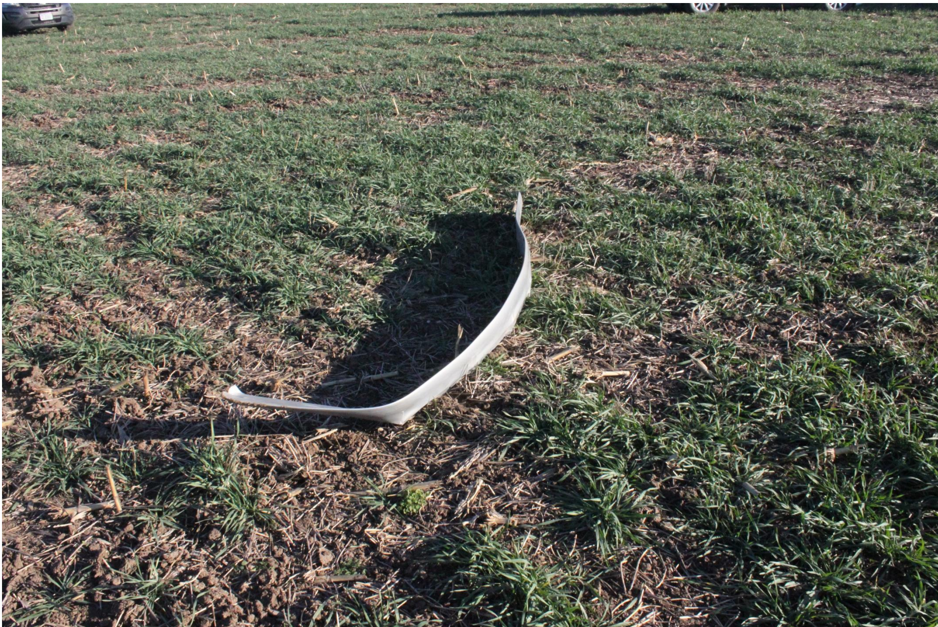
Photo 3 – View of the accident gyroplane displaced rotor blade (Photo courtesy of the FAA)
