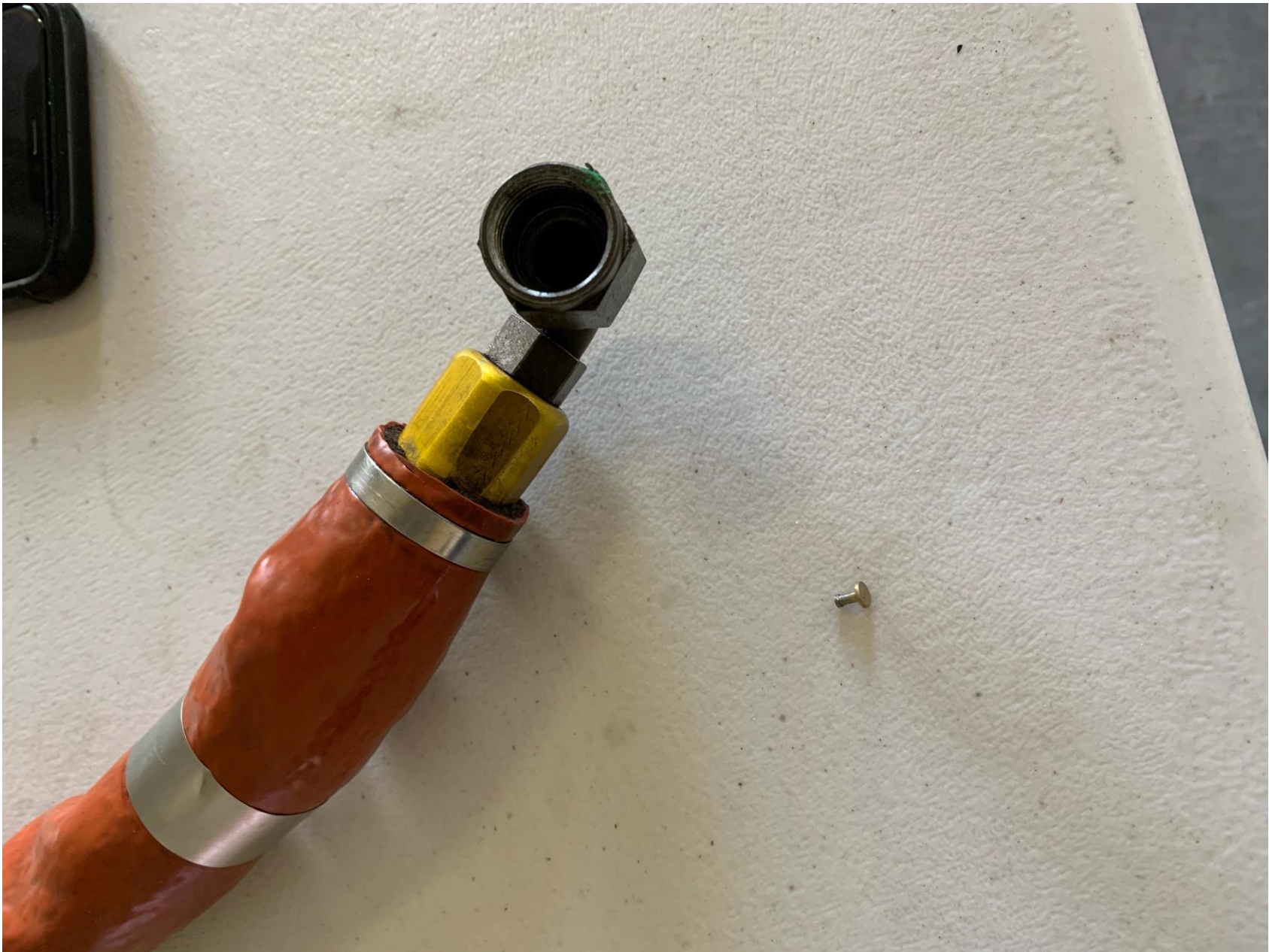
Photo 4 – View of the fuel line and pin from the accident fuel pump (Photo courtesy of the FAA)
