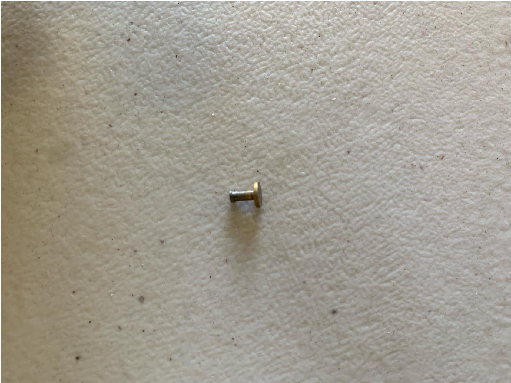
Photo 5 – View of the accident fuel pump pin that was found in the fuel line (Photo courtesy of the FAA)
