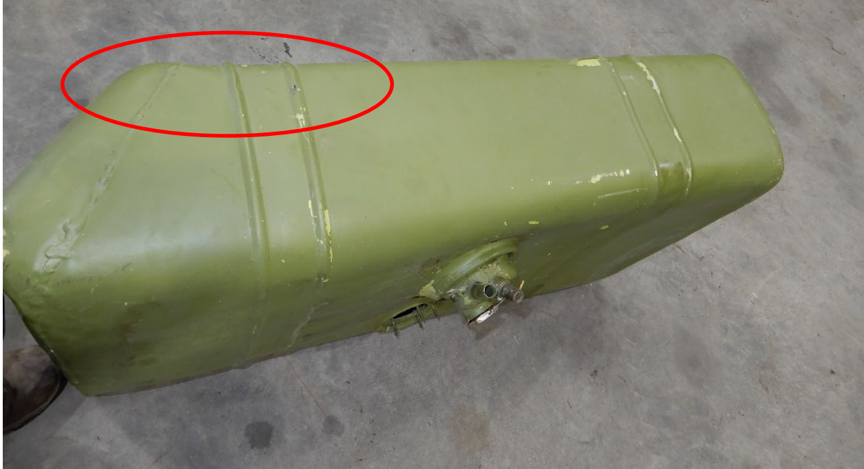
Figure 7 - Center Fuel Tank (Area of hydraulic deformation in red circle)
