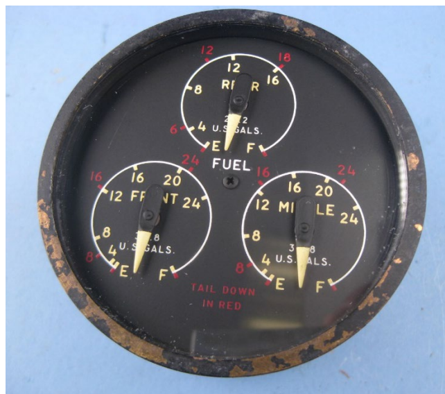
Figure 12 - The Fuel Quantity Indicator, as recovered.
