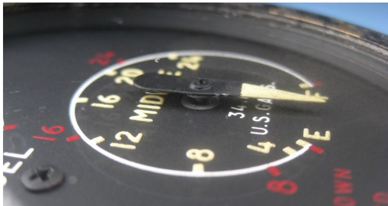
Figure 14 -The indication area of the MIDDLE fuel tank, with no impact marks noted.
