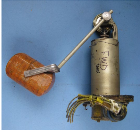
Figure 8 - Fuel Quantity Sensor removed from the Front Fuel Tank.
