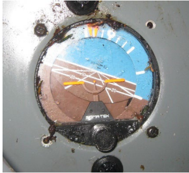
Figure 10 - Attitude Indicator, as noted after airplane recovery.
