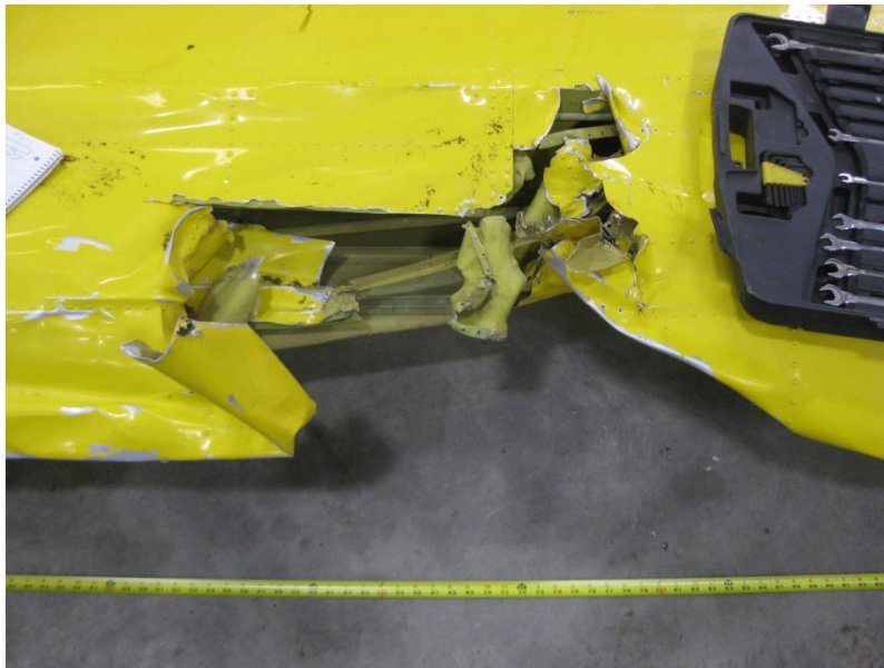
Figure 20 - Left wing. Note the angled impact marks.
