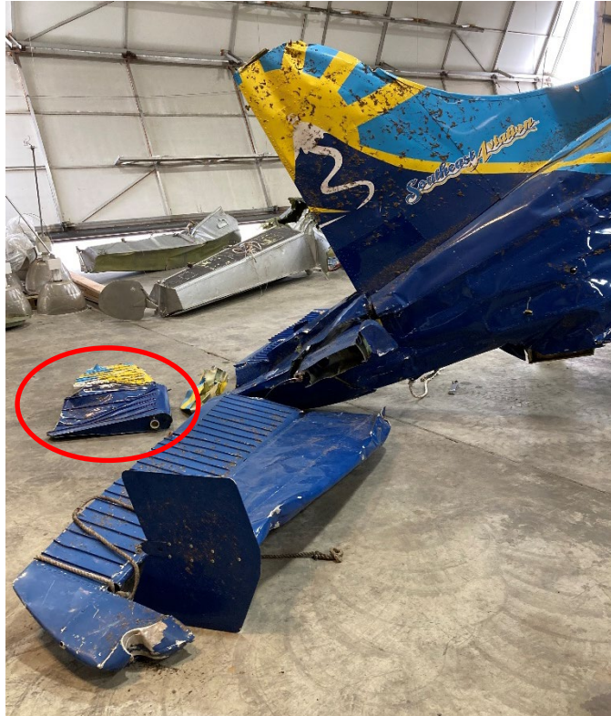
Figure 18 - Tail Section of Airplane, showing right horizontal stabilizer, vertical stabilizer, and rudder (separated, circled in red). (Photo courtesy of the FAA)
