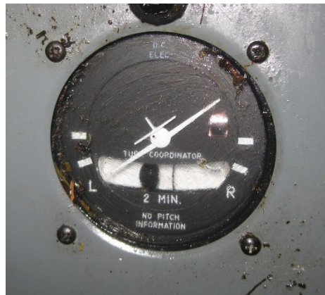
Figure 11 - Airplane Turn Coordinator, left wing down indication.
