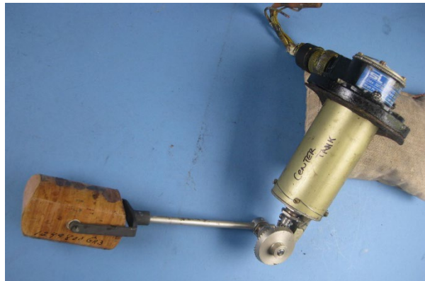
Figure 9 - Fuel Quantity Sensor removed from the Center Fuel Tank.
