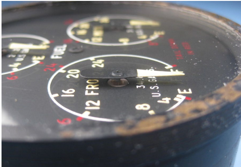
Figure 13 - The indication area of the FRONT fuel tank, with no impact marks noted.
