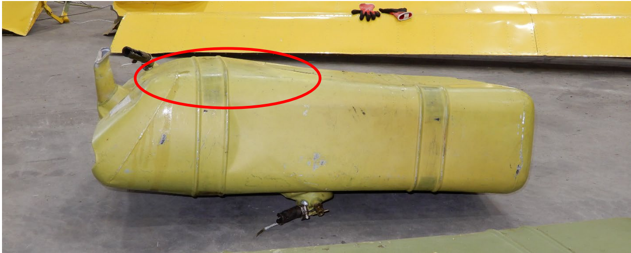
Figure 6 - Front Fuel Tank (Area of hydraulic deformation in red circle)
