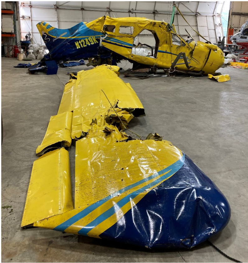
Figure 21 - Right Wing and right side of fuselage, during the airplane examination. (Photograph courtesy of the FAA)
