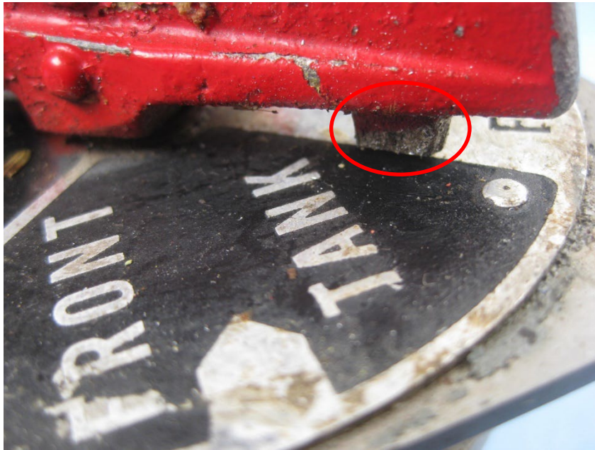
Figure 2 - Fuel Selector Panel, FRONT TANK Selection Area. Note the selector handle tab circled in red.
