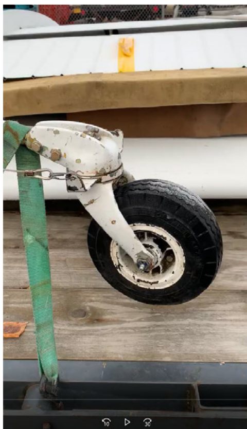
Photo 2 - Accident airplane's tailwheel.
