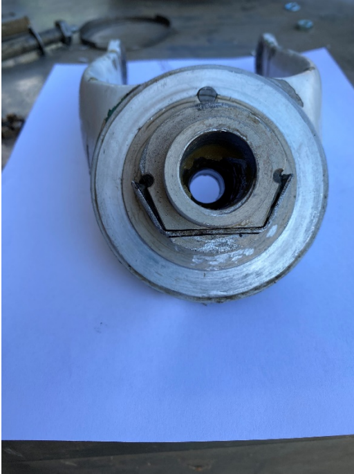
Photo 7 - Compression spring in its respective attach point. Note, no spacer present.
