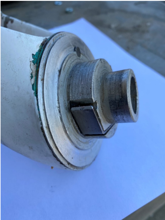
Photo 8 - Compression spring's sharp and damaged spring end.
