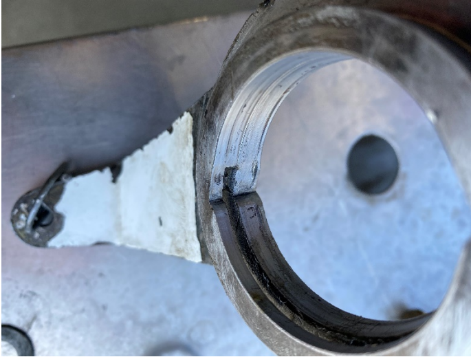
Photo 5 - Tailwheel steering arm's scored and damaged inside radius.
