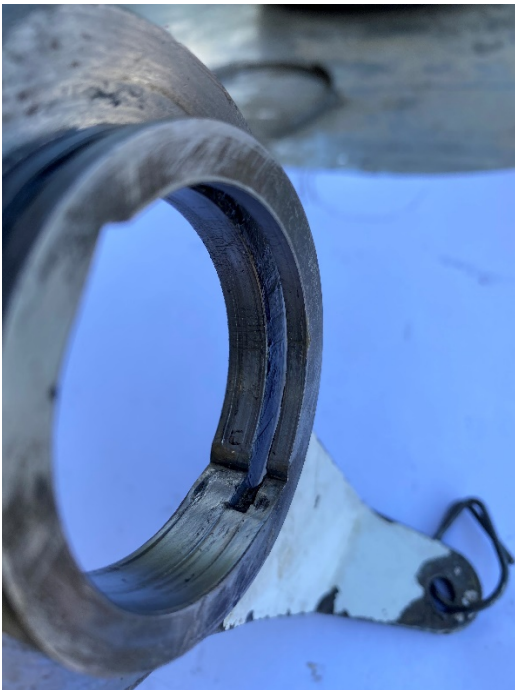
Photo 6 - Tailwheel steering arm's scored and damaged inside radius.
