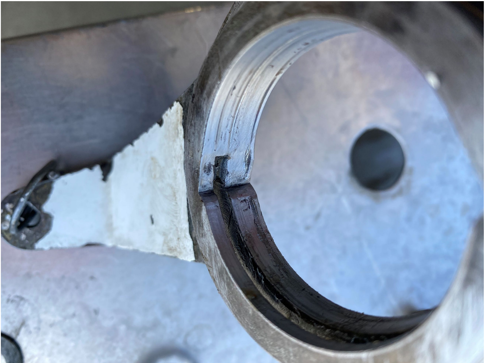
Photo 2 – Tailwheel steering arm's scored and damaged inside radius.
