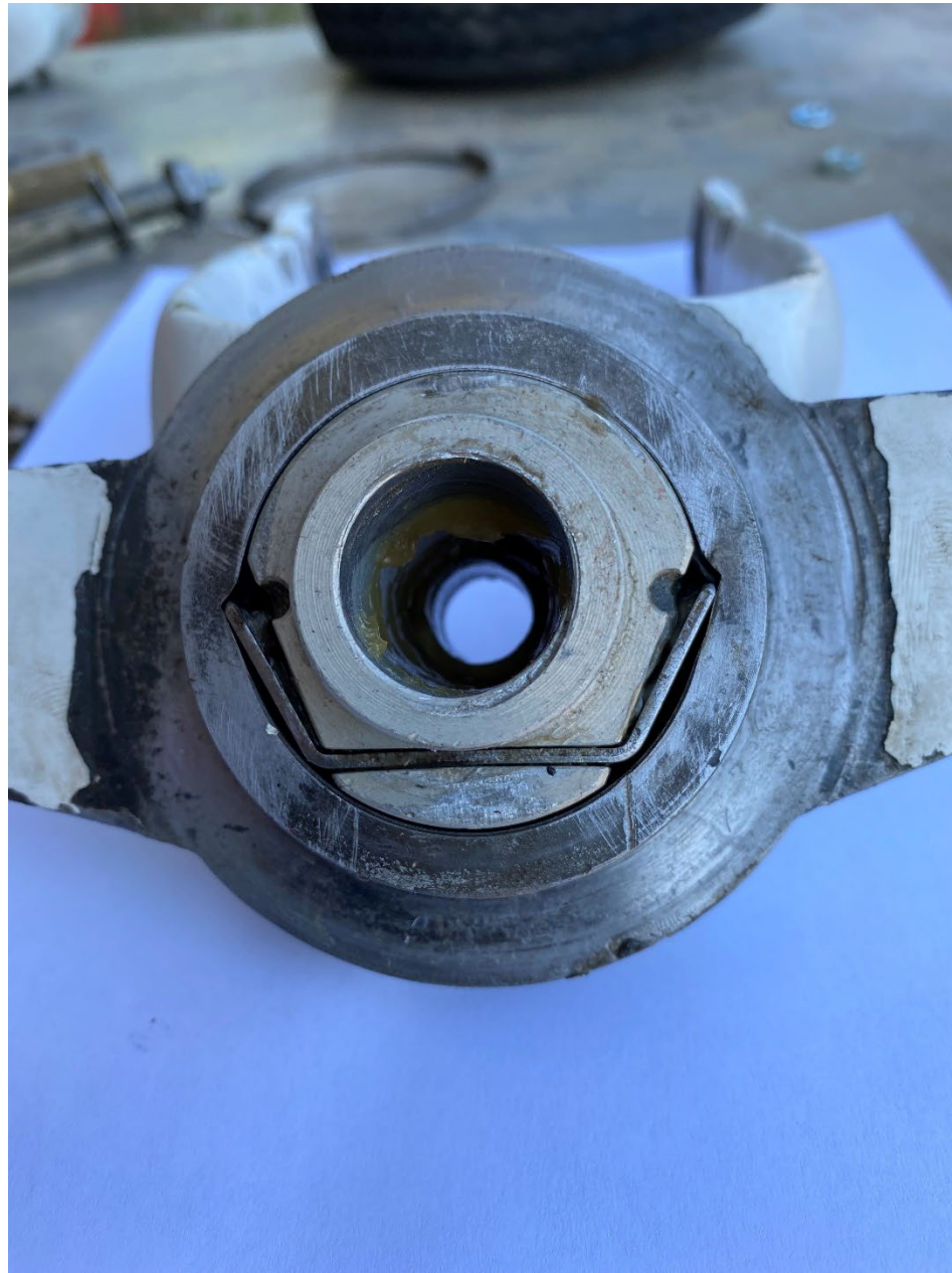
Photo 4 - Compression spring in its respective attach point. Note, no spacer present.
