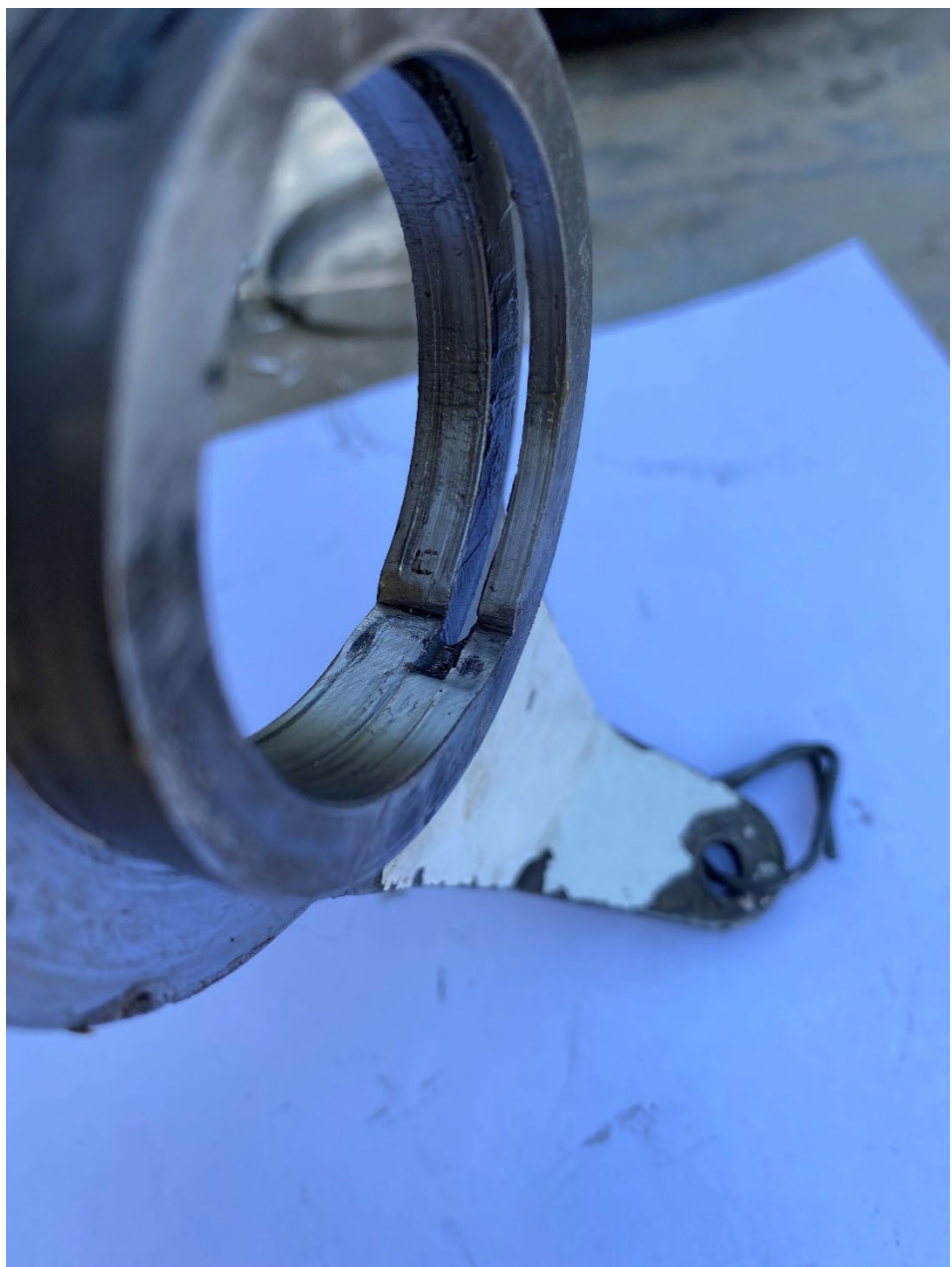
Photo 3 – Tailwheel steering arm’s scored and damaged inside radius.
