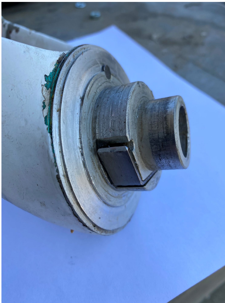
Photo 5 - Compression spring's sharp and damaged spring end.
