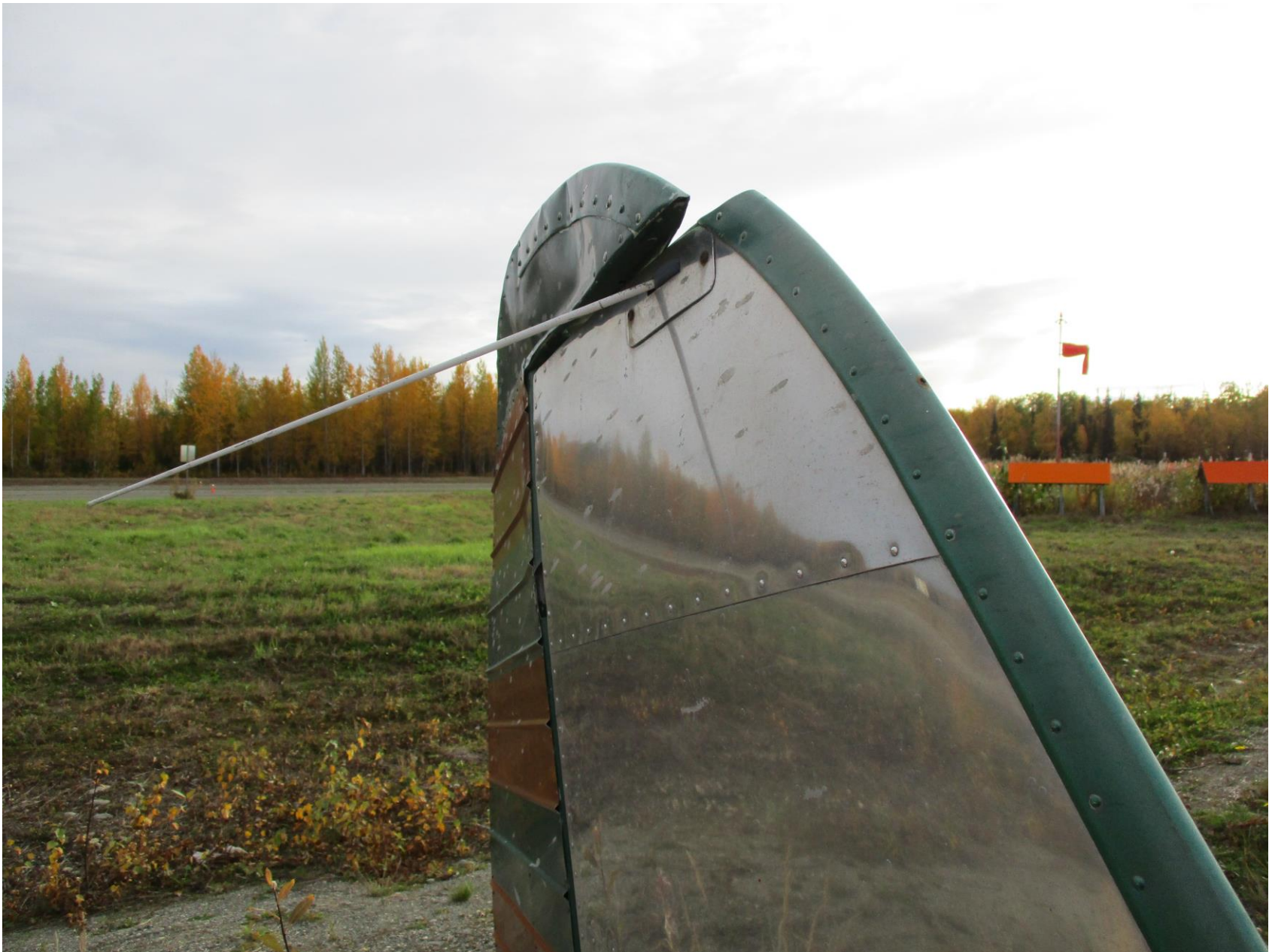
Photo 4 – View of empennage damage (Photo courtesy of the FAA)
