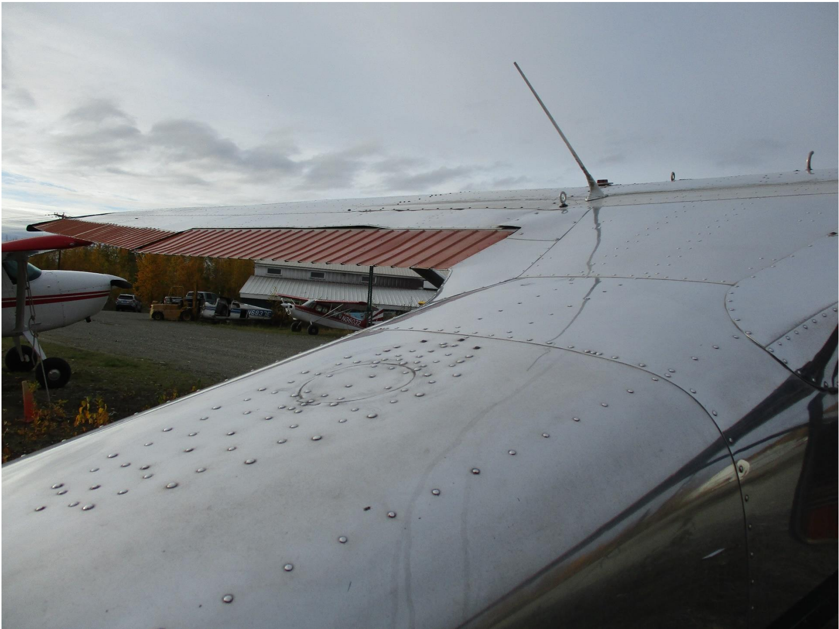
Photo 3 – Top view of damaged left wing (Photo courtesy of the FAA)
