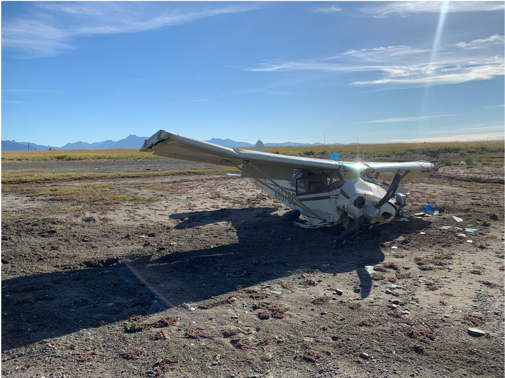
Photo 2 - Right wing and fuselage damage. (Photograph courtesy of the Alaska State Troopers.)
