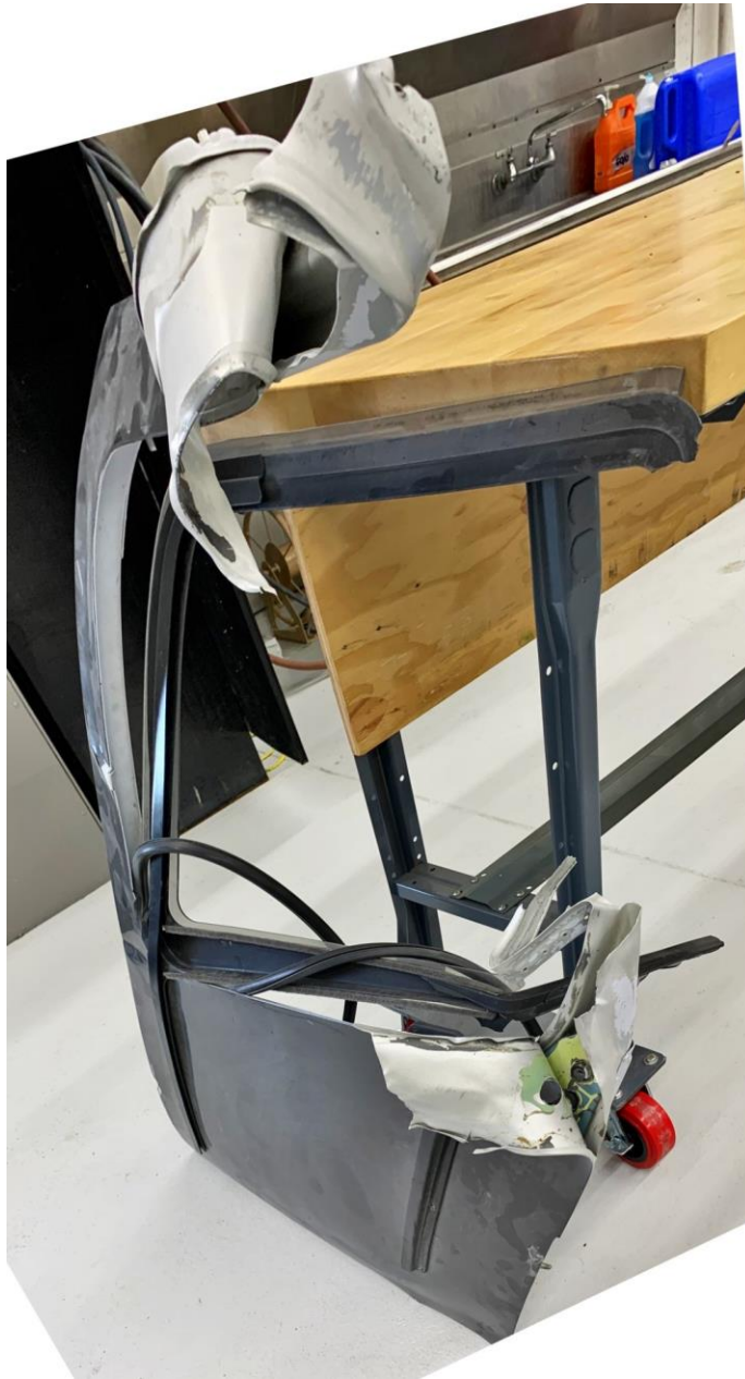
Photo 4 – Damaged left sliding door (Photo courtesy of the Operator)
