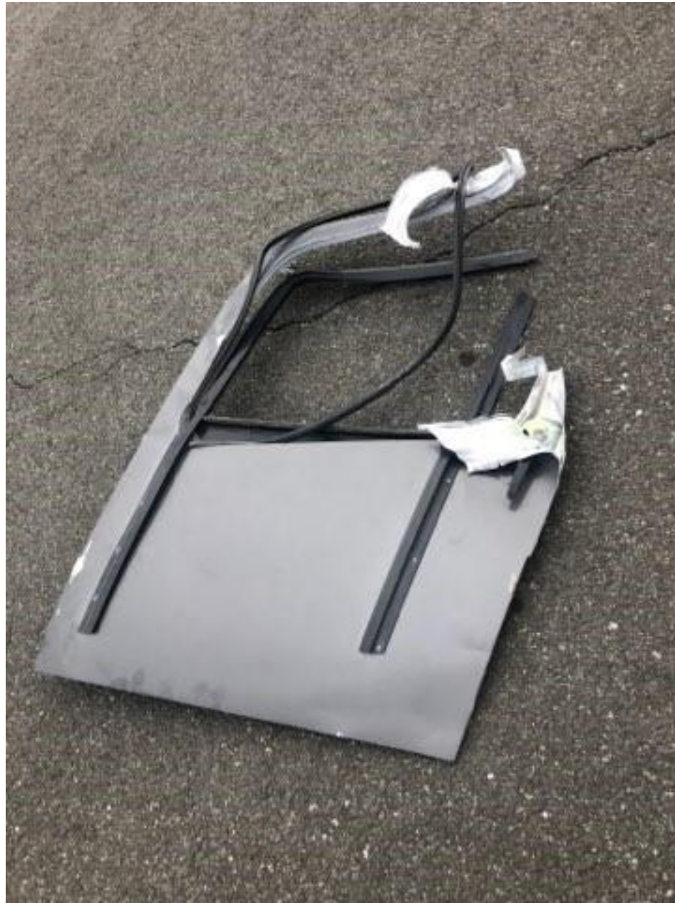
Photo 3 – Damaged left sliding door (Photo courtesy of the Operator)
