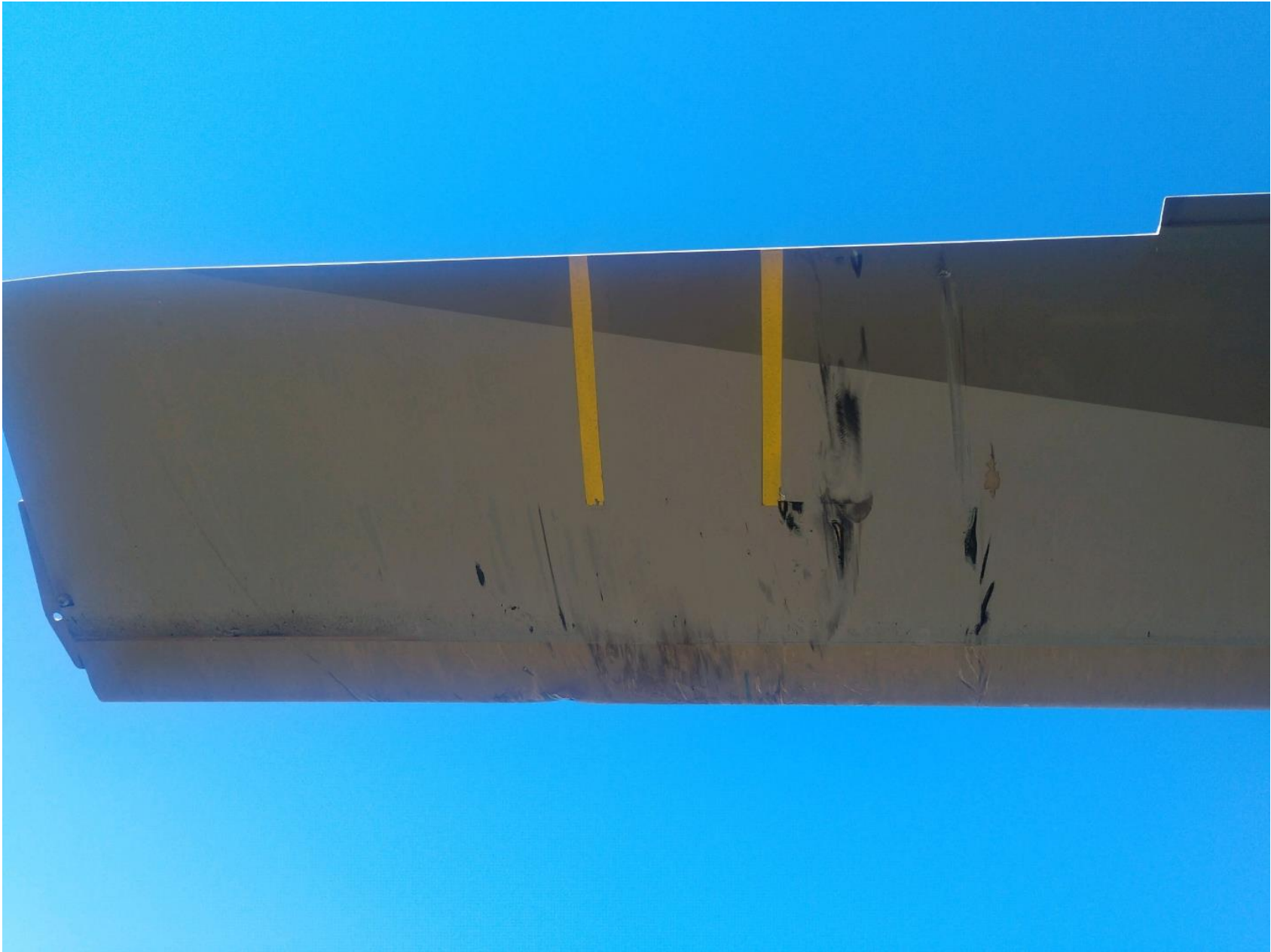
Photo 1 – View of damaged main rotor blade (Photo courtesy of the Operator)
