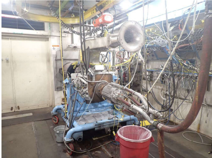
Figure 25. Engine S/N LE-46018, Installed in Test Cell
