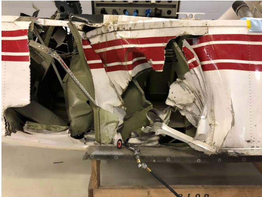
Figure 1 - Left float damage before trimming.
