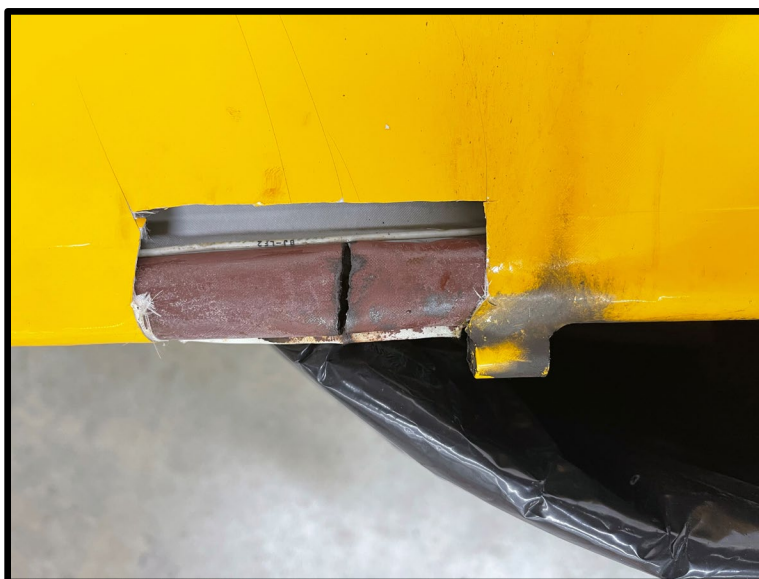
Figure 2-PA-18 fractured rudder post.
