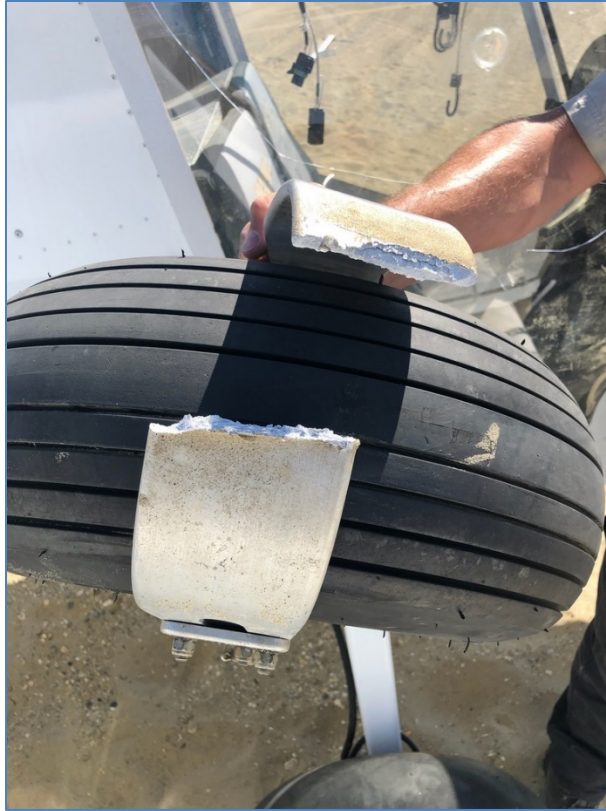
Figure 1. Fractured nosewheel fork
