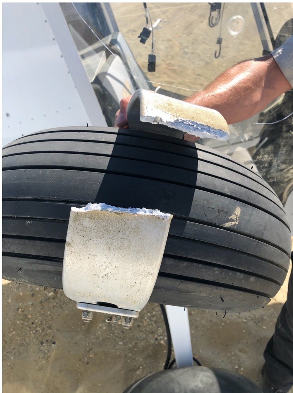
Photo 2 - Fractured nosewheel fork. (Courtesy of the owner.)
