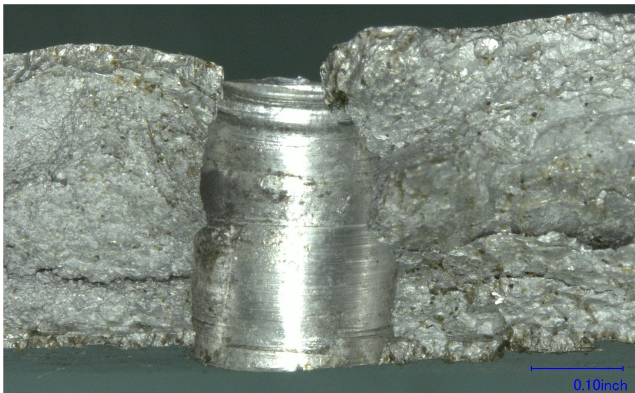
Figure 7 – A closer view of the fracture surface features around the bolt hole in Figure 6a.
