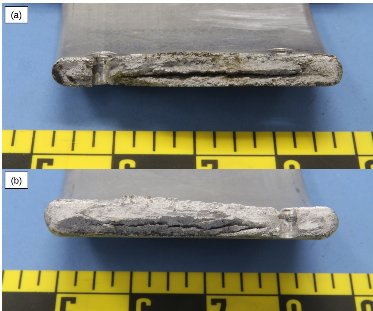
Figure 6 – The mating left side fractures from Figure 1 through 3, showing the (a) the left fracture surface of the middle piece and (b) outer left piece fracture surface.
