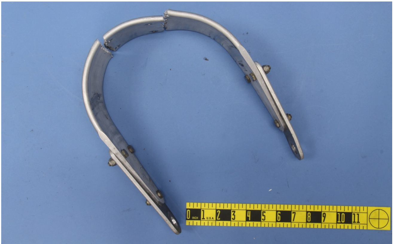
Figure 2 – The three fractured fork pieces, positioned in their locations at fracture, viewed from the side.
