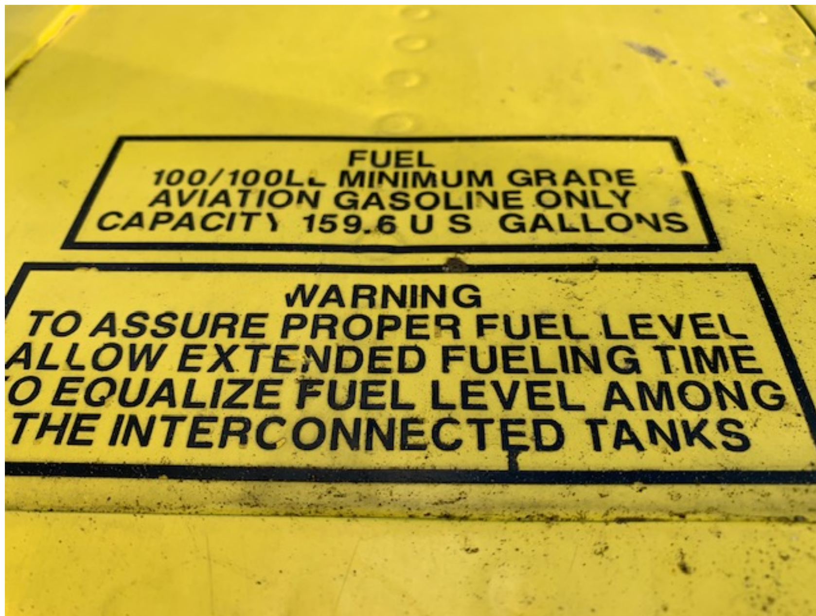
Photo 3 – Fuel placard on accident airplane located near fueling port.
