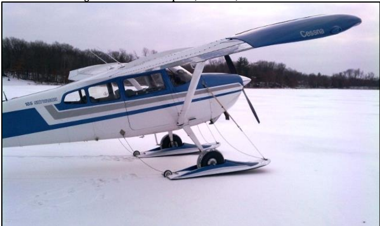
Figure 2: Exemplary Wheel/Ski-Equipped Cessna A185E
