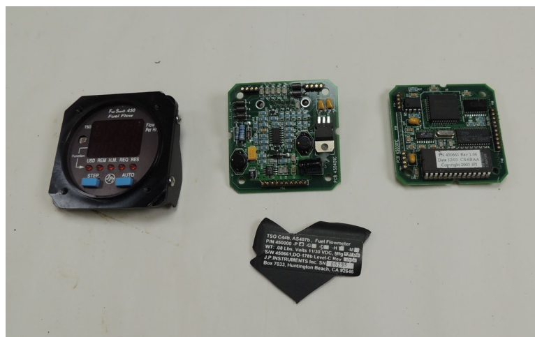
Figure 2. Photo of damaged JPI FS-450
