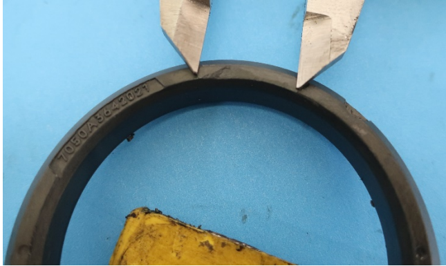
Photo 4 - No. 1 outer bearing showing abrasion mark on the outer face.
