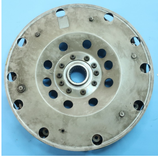
Photo 2 - Fenestron hub as received
