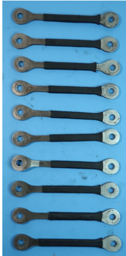
Photo 6 - Torsion bars, back sides
