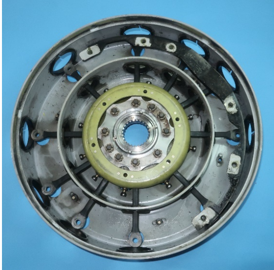
Photo 1 - Fenestron hub as received
