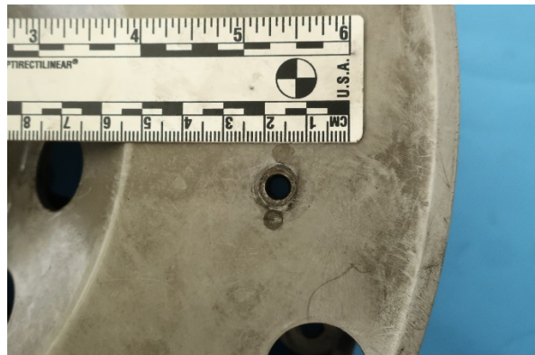
Photo 3 - Closeup of missing balance weight location.
