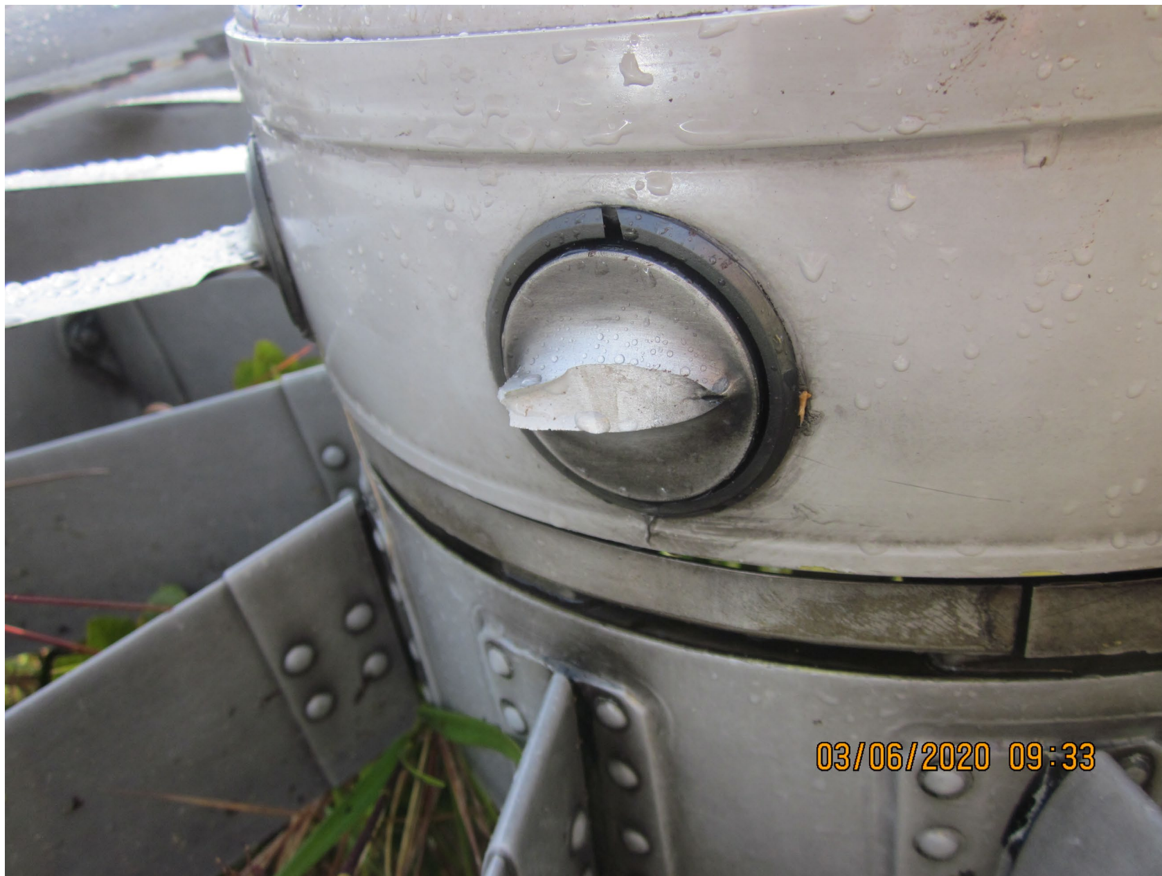
Photo 4 – Accident helicopter's ruptured fenestron blade root. Photo provided by unknown.
