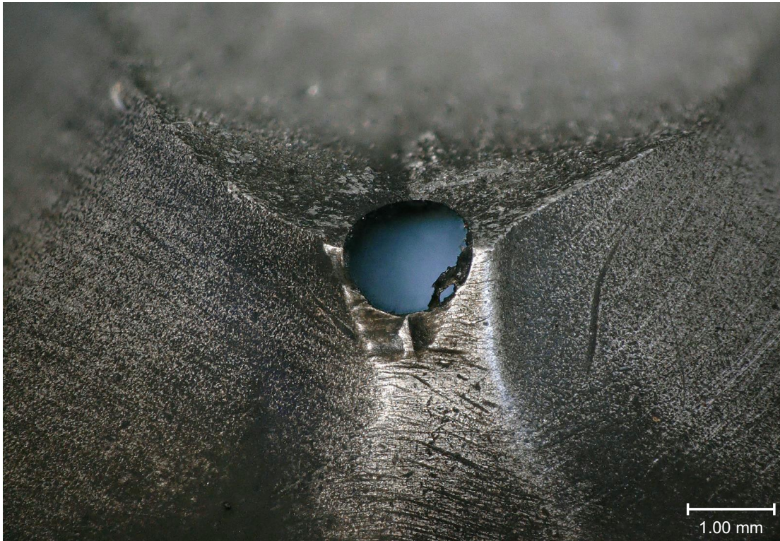
Figure 9: View along the longitudinal axis of the drain hole. Backlighting from a fiber optic light is visible through the passage, consistent with no obstruction.
