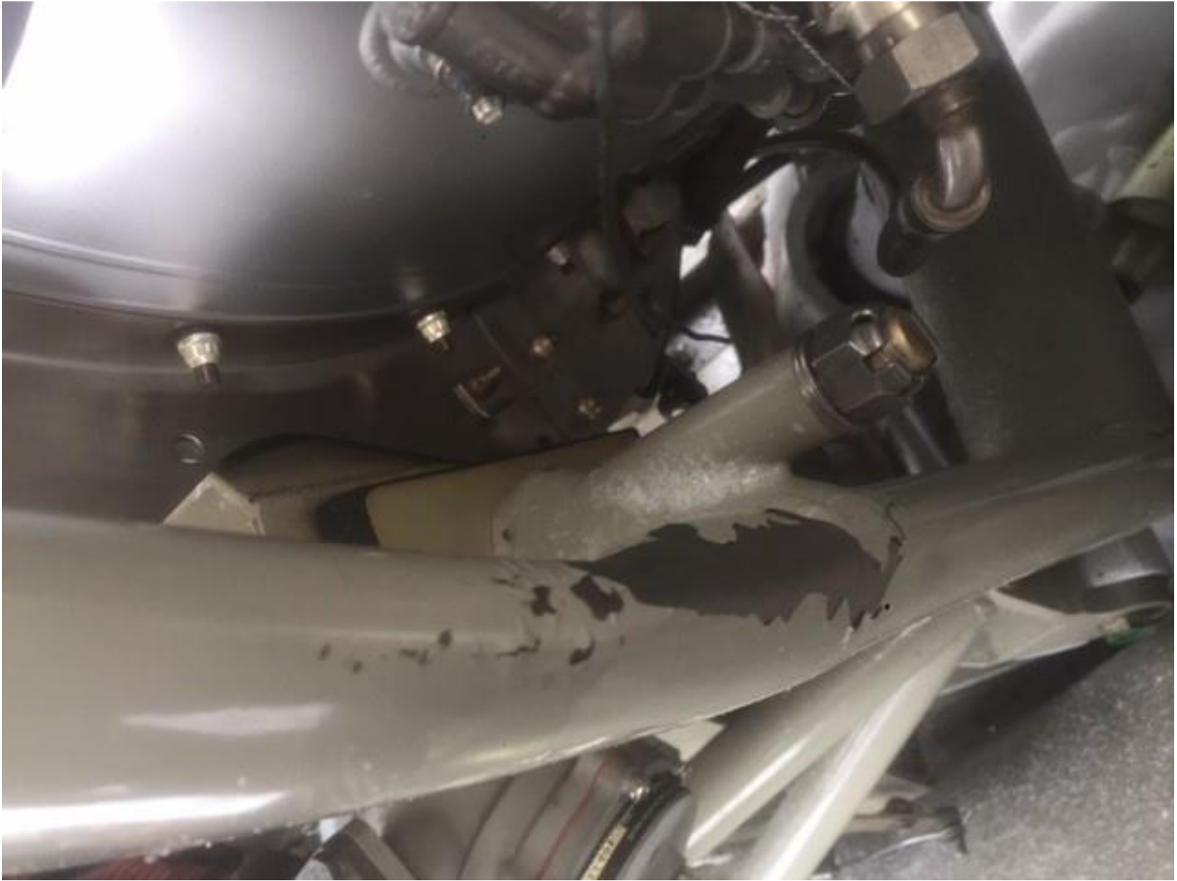
Photo 2 – View of damaged engine mount (Photo courtesy of unknown)
