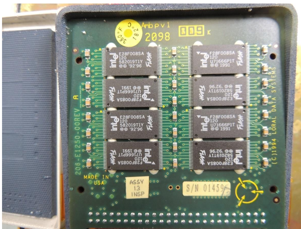
Figure 1. CSMU interior showing minor water intrusion.
