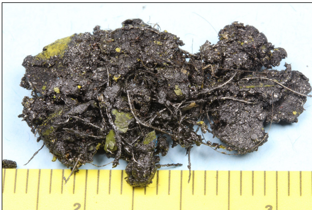
Figure 9. Sample of deposits collected from the rudder pulley area. Black deposits were mixed with chips of green primer, metal shavings, and wire fragments.
