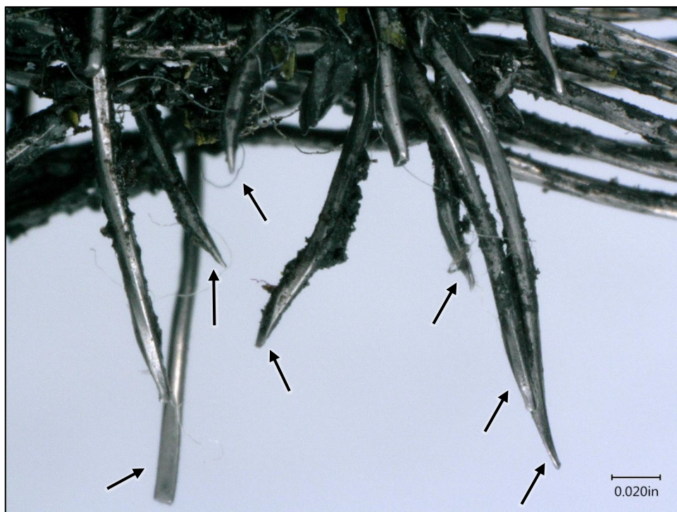
Figure 4. Closer view of individual wires from strands that were bent back. The ends of many wires from the outer strands were worn to a chisel-like end such as the wires indicated with unlabeled arrows.
