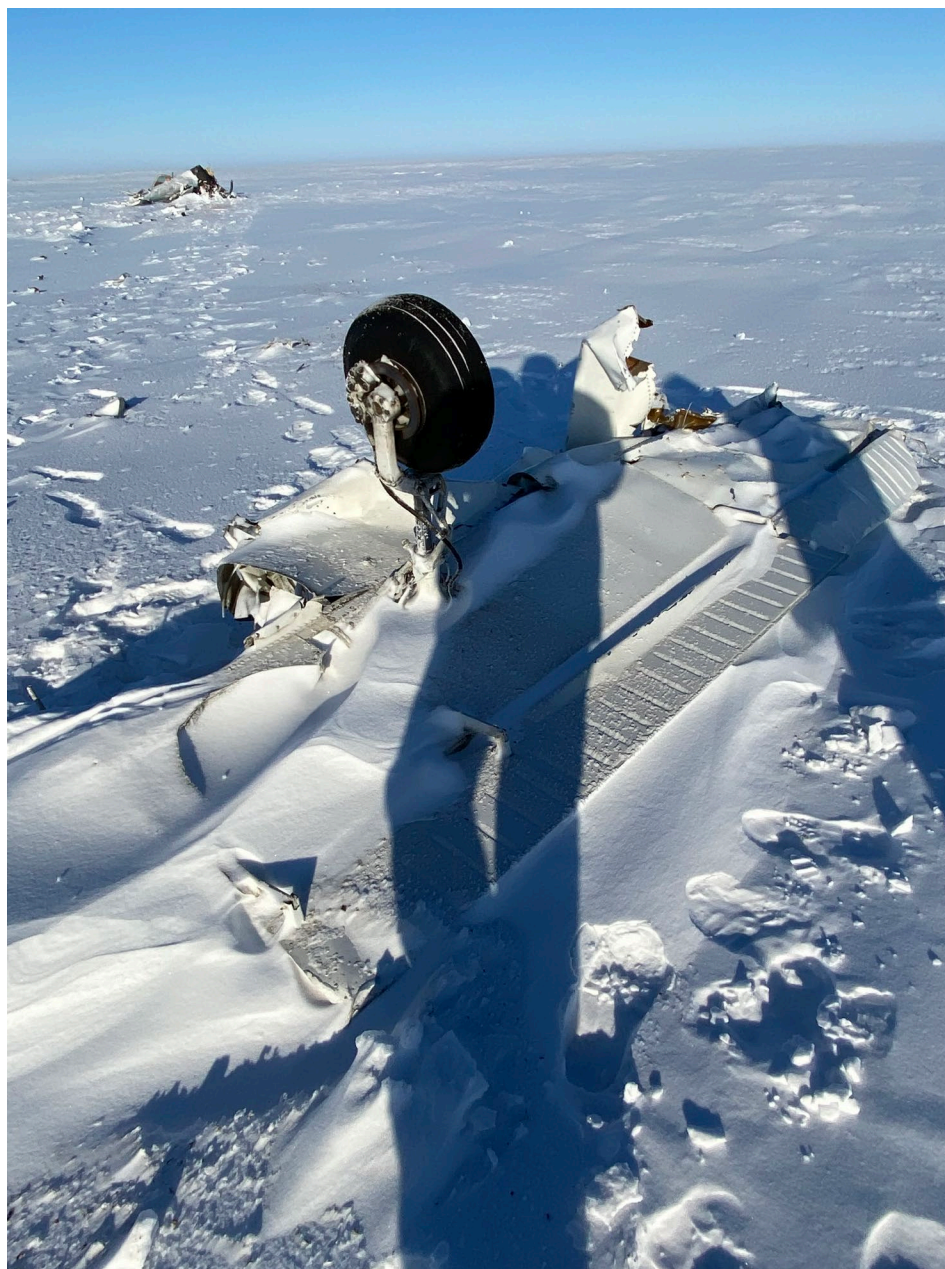
Photo 4 - Photo of accident airplane's severed right wing in foreground, and main wreckage in background.
