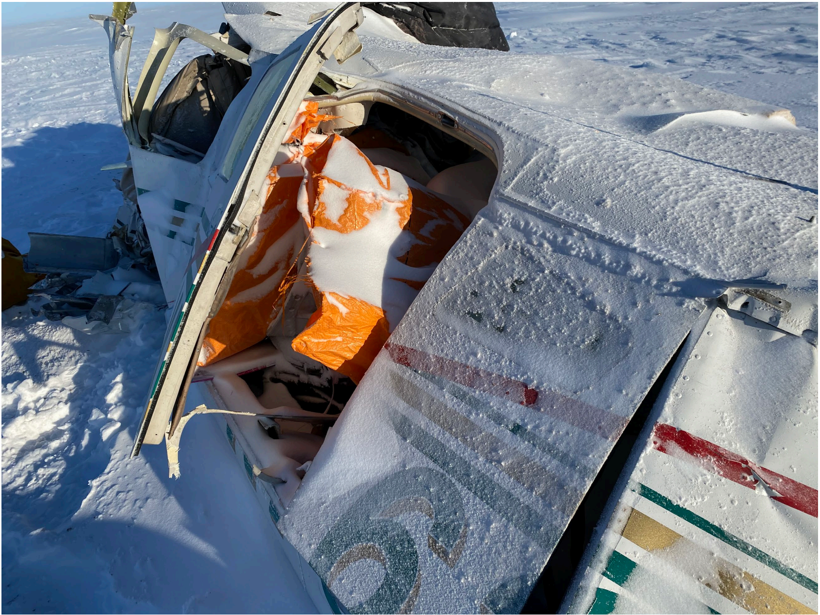
Photo 3 - Photo of accident airplane's left side, cargo door area.
