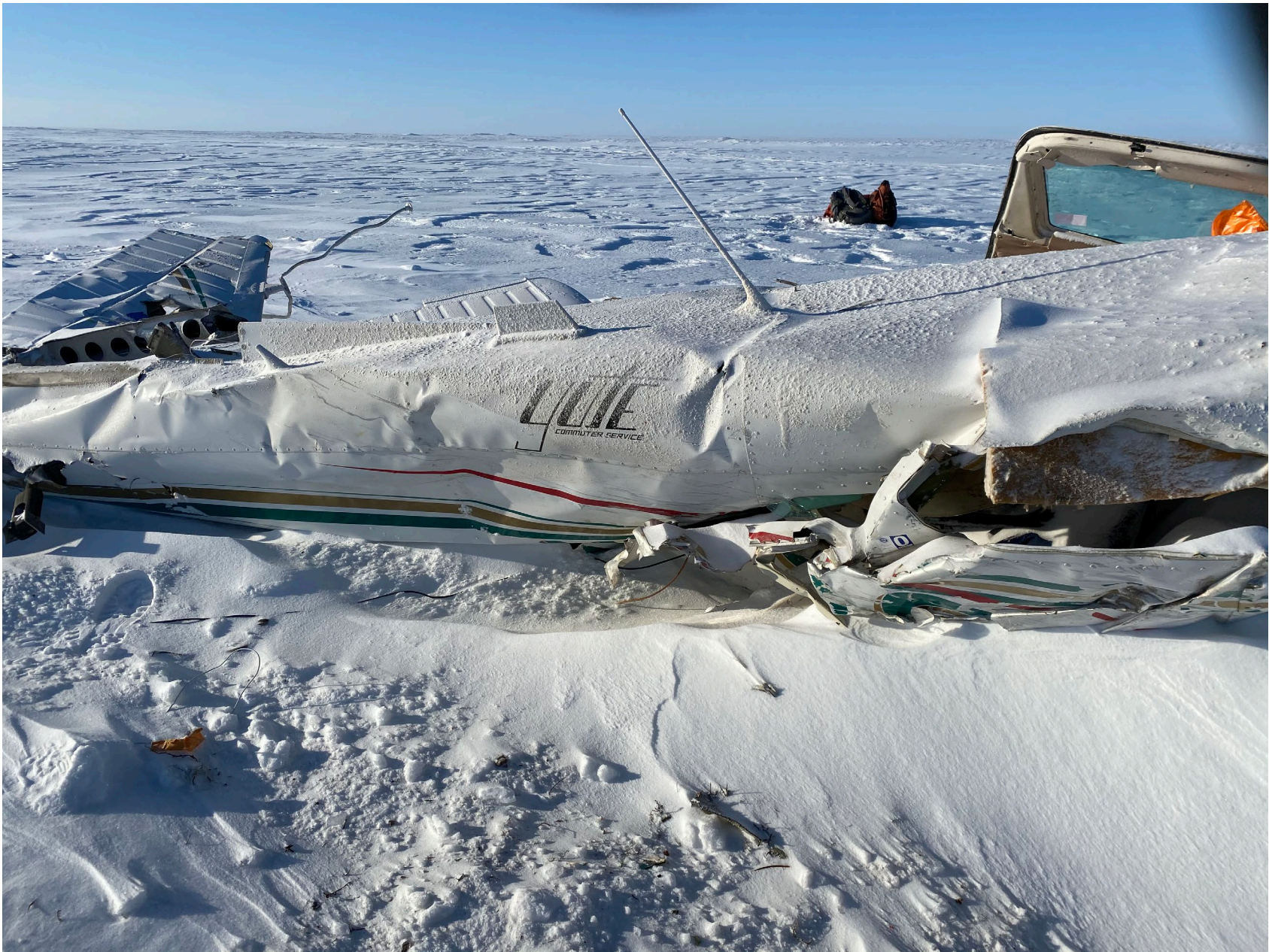
Photo 5 -Photo of accident airplane's empennage and aft fuselage. Photo taken from right side.
