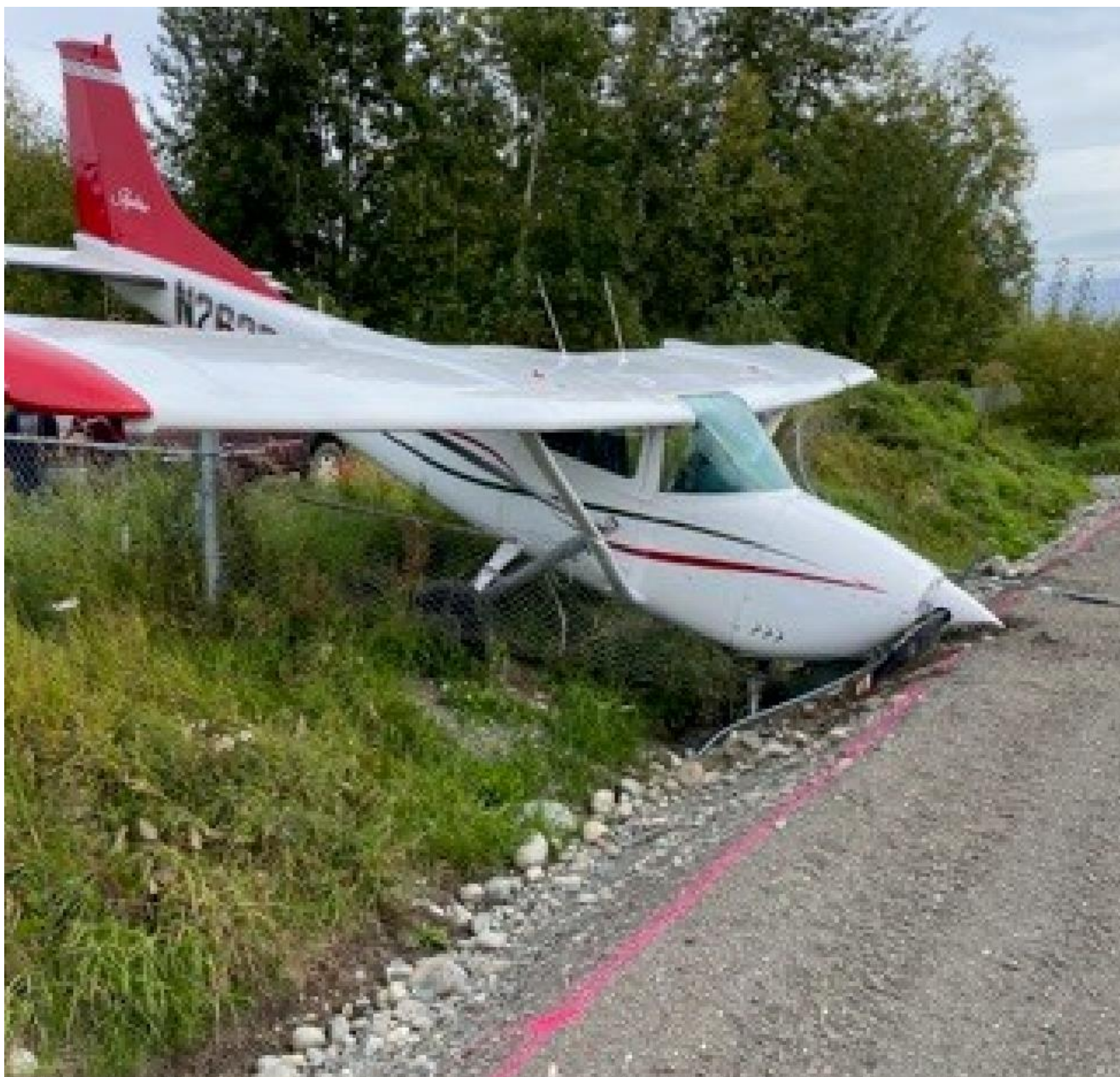
Photo 2 – View of damaged right-wing lift strut (Photo courtesy of the Alaska State Troopers)
