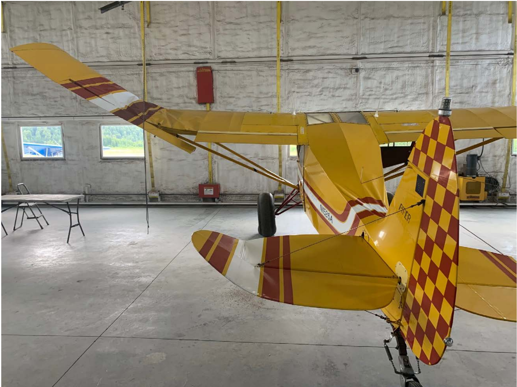
Photo 1 – N1526A PA-20 exhibiting substantial damage to the left wing and horizontal stabilizer. (Photograph courtesy of the Federal Aviation Administration.)
