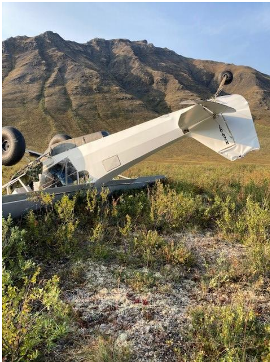
Photo 1 – View of airplane inverted and damaged rudder (Photo courtesy of the pilot)
