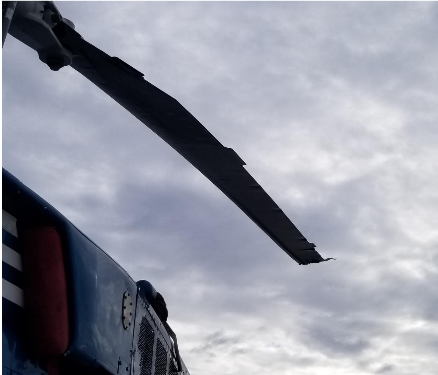
Photo 2 – Additional view of main rotor blade damage (Photo courtesy of the operator)
