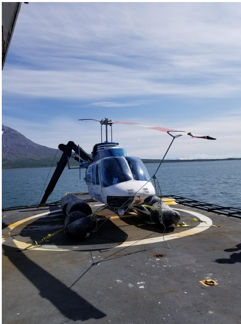
Photo 1 – View of main rotor blade damage (Photo courtesy of the operator)
