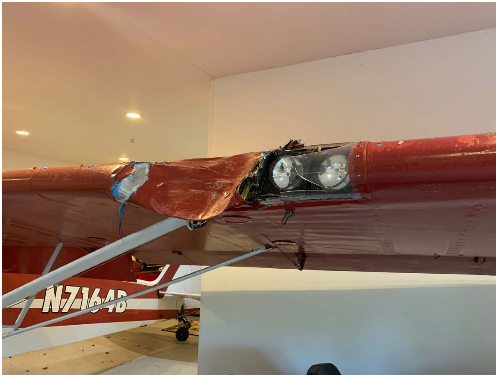
Photo 2 – Accident airplane's damaged left wing.
