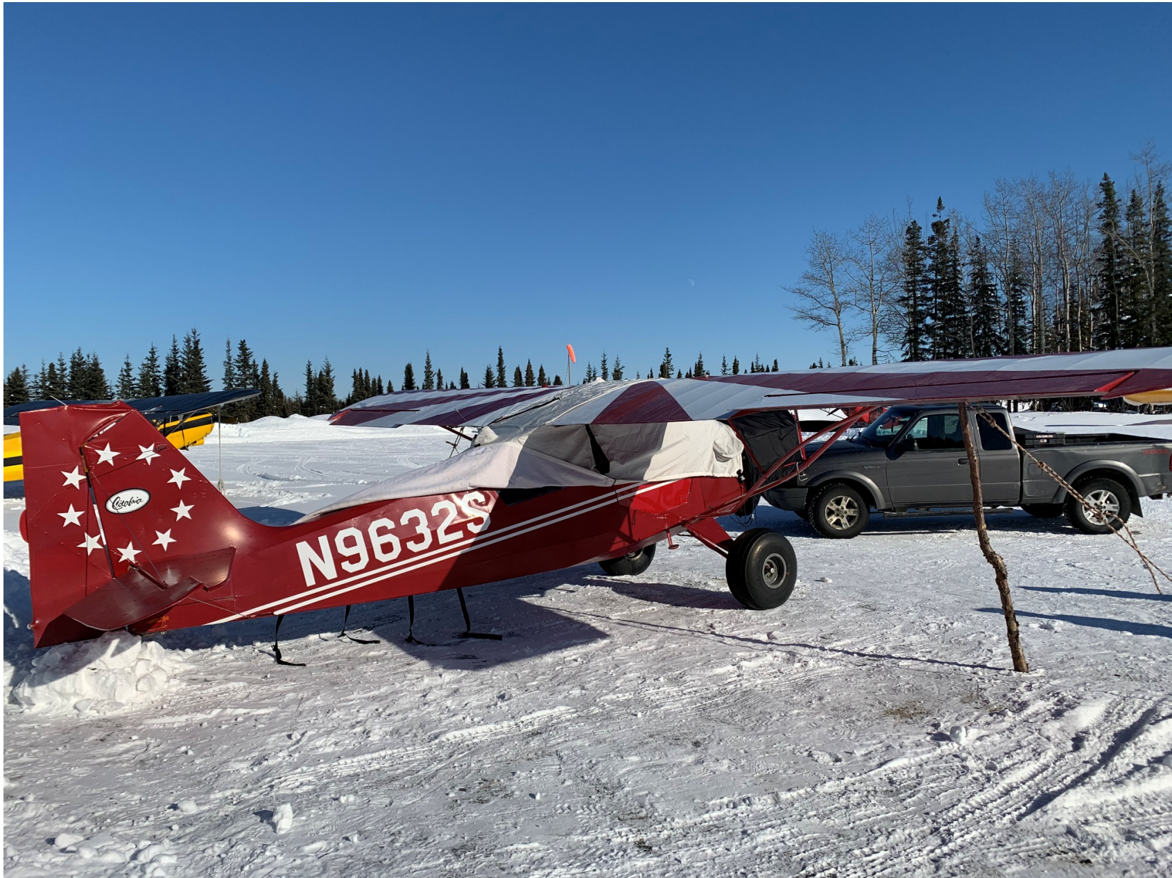
Photo 2 - Accident Airplane's Right Side, Showing Damage to Empennage and Wings (FAA Photo)
