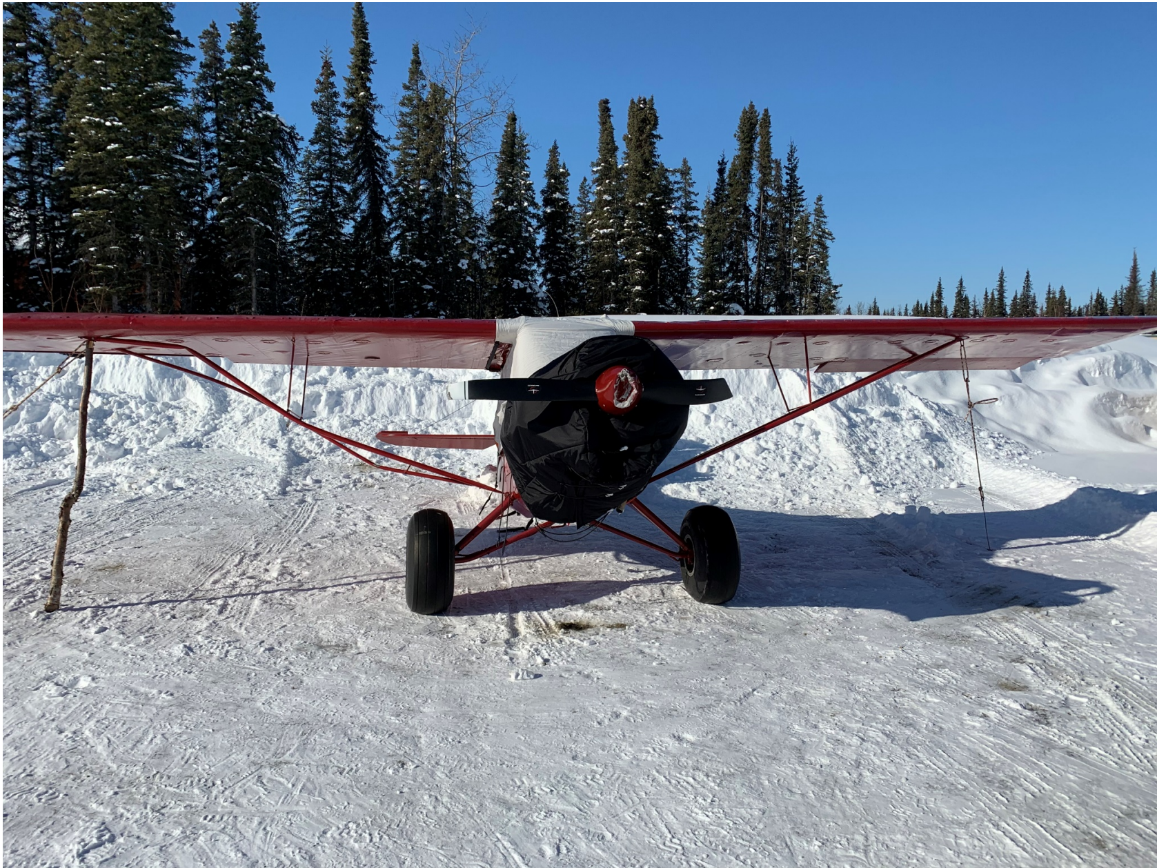
Photo 1 – Accident Airplane’s Nose, Showing Damage to Propeller and Right Wing Lift Struts (FAA Photo)
