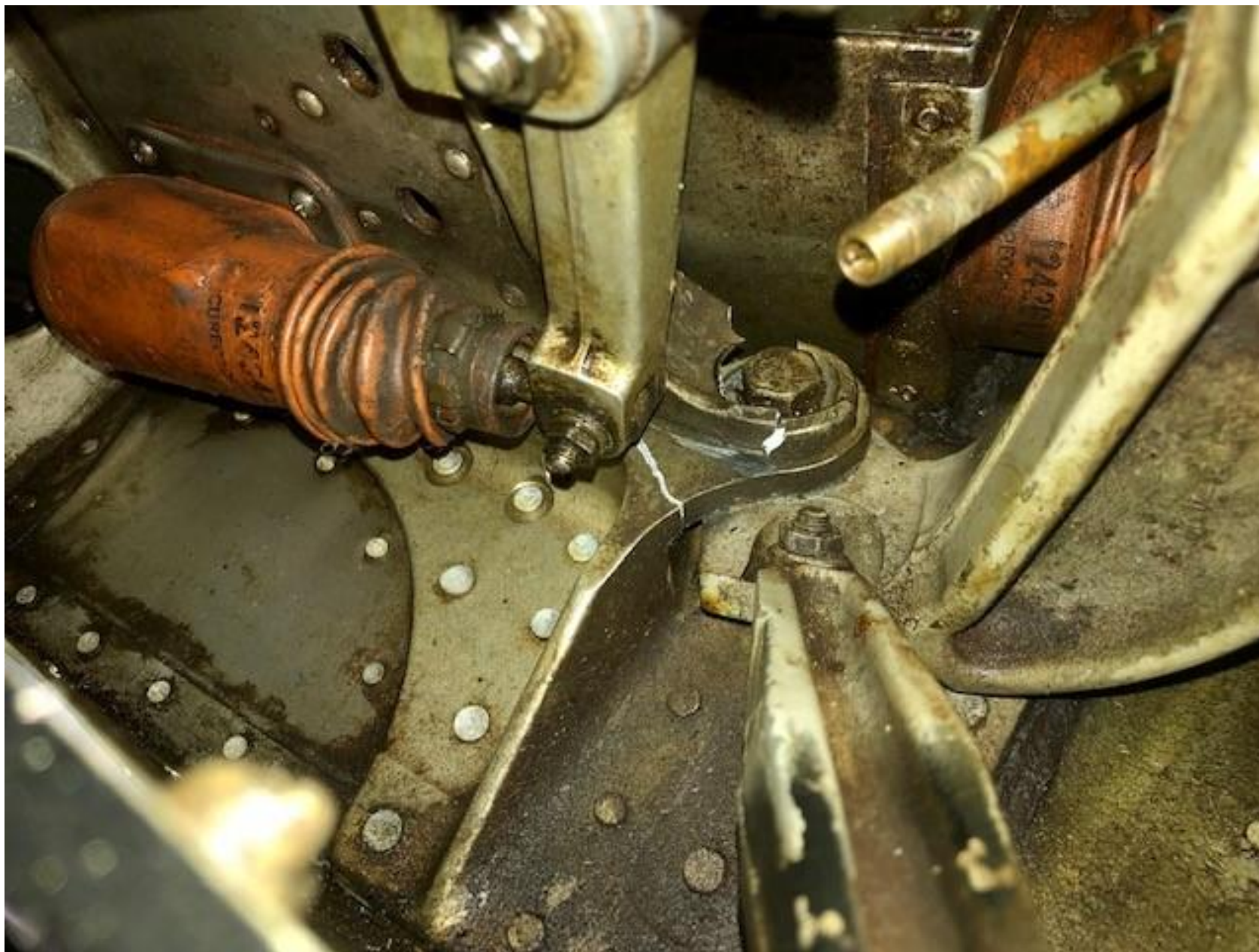
Photo 2 – View of damaged fuselage fitting (Photo courtesy of the mechanic)
