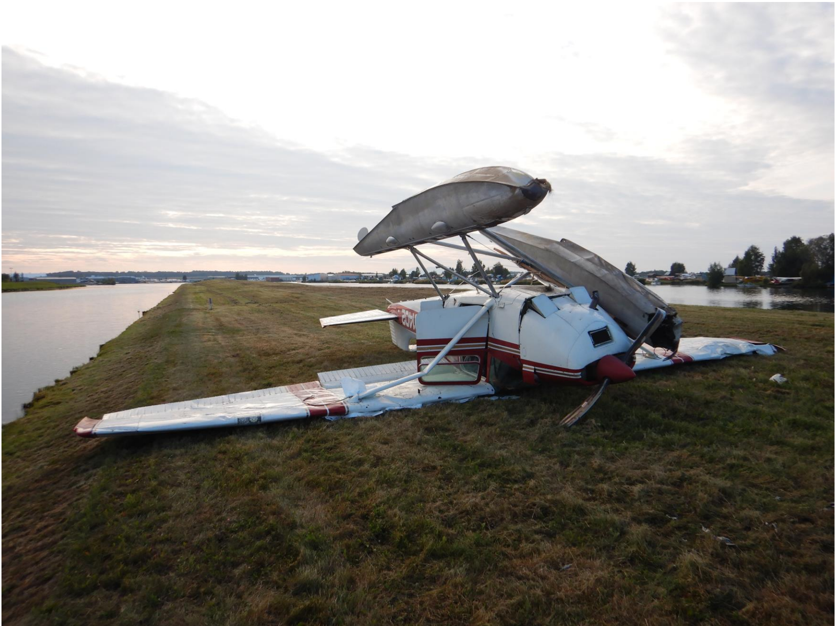
Photo 4 – Front view of damaged wings, lift strut, and empennage (Photo courtesy of the NTSB)
