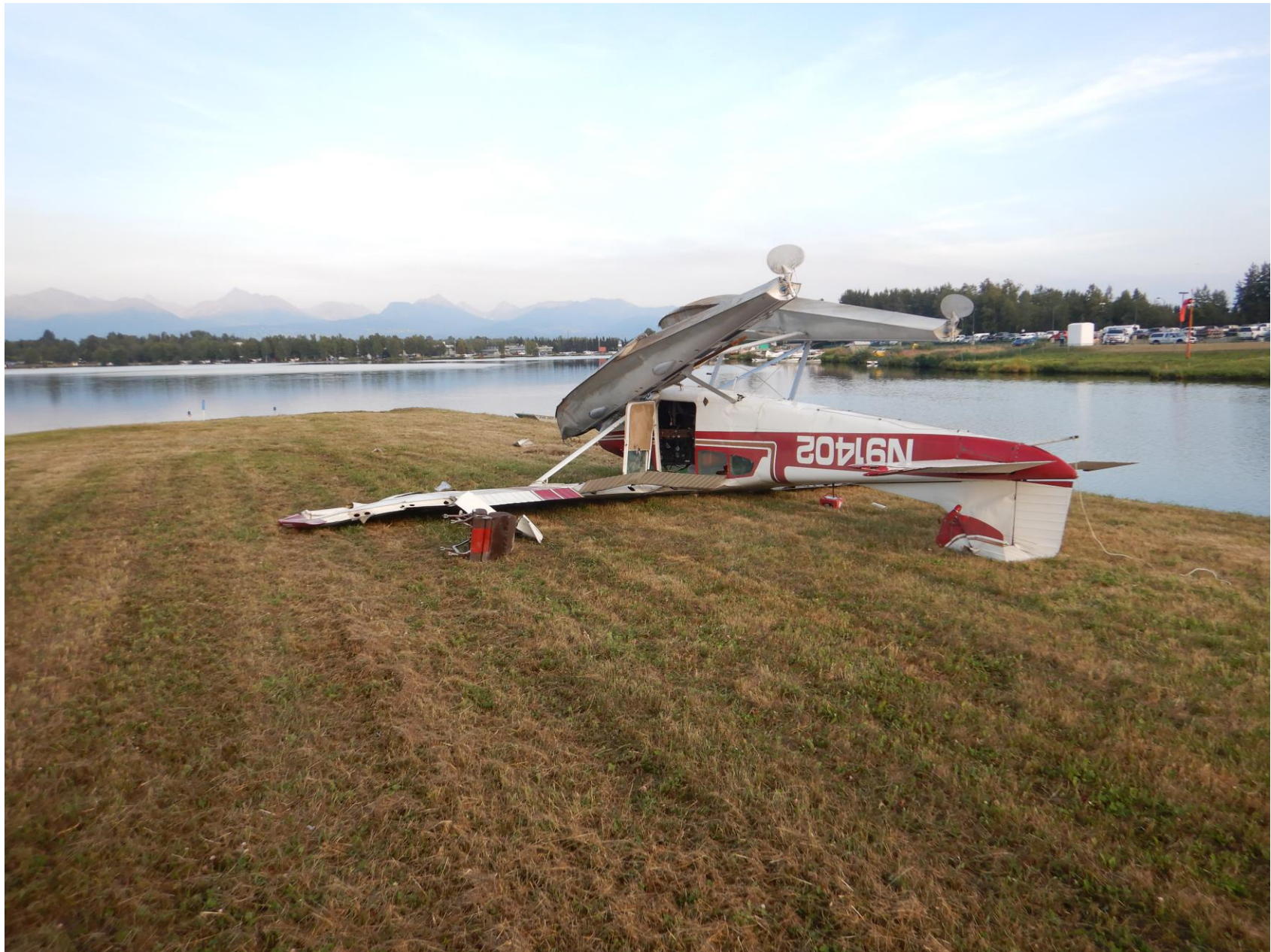
Photo 3 – Rear view of inverted airplane and damaged empennage (Photo courtesy of the NTSB)
