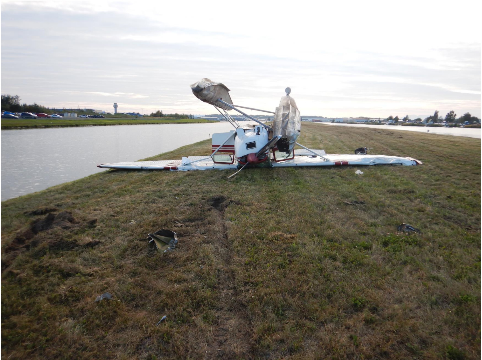
Photo 2 – View from front of inverted airplane with damaged wings and lift strut (Photo courtesy of the NTSB)
