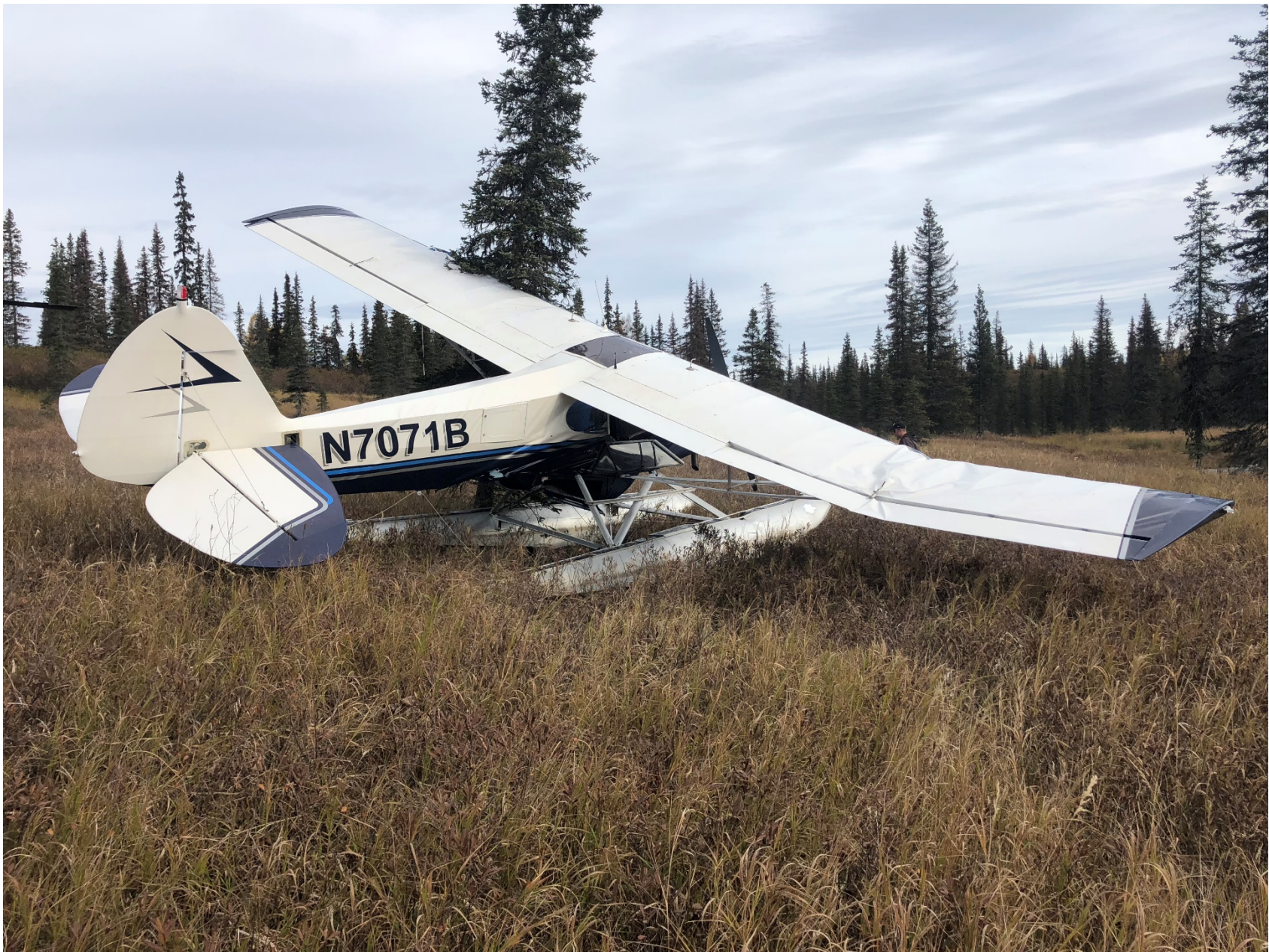
Photo 1 – N7071B Piper PA-18 at the accident scene exhibiting substantial damage to the fuselage and right wing. (Photograph courtesy of the owner.)
