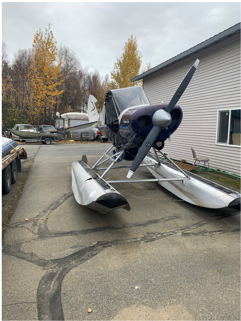
Photo 2 - Wreckage with the wings removed before the engine examination.
