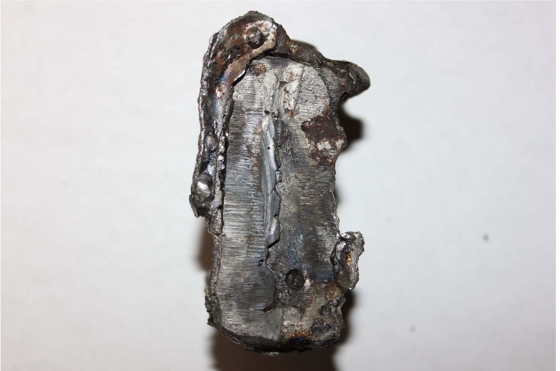
Photo 4 – Separated landing gear fitting.
