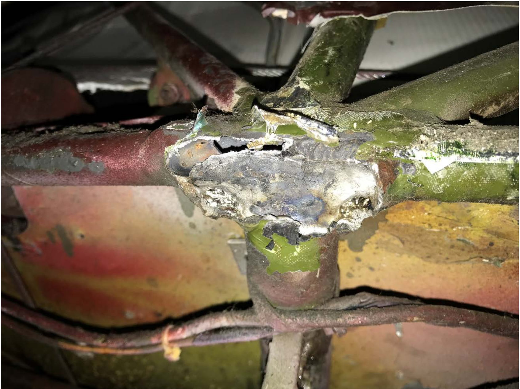
Photo 3 – Fuselage where landing gear fitting separated.
