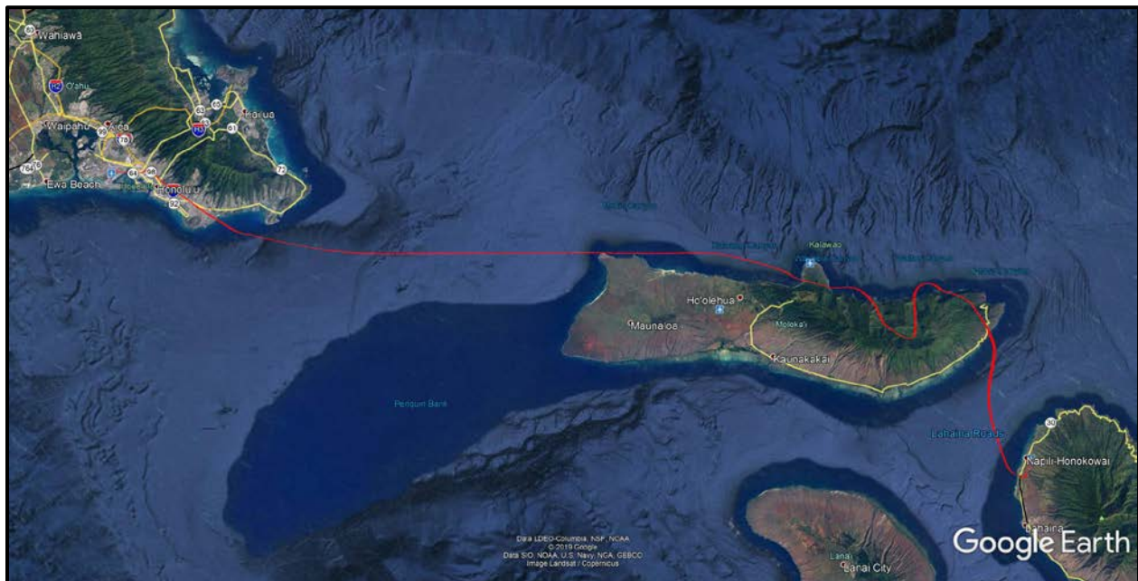
Figure 2: Mokulele Airlines Flight 504 Ground Track Recorded on Recovered G1000
