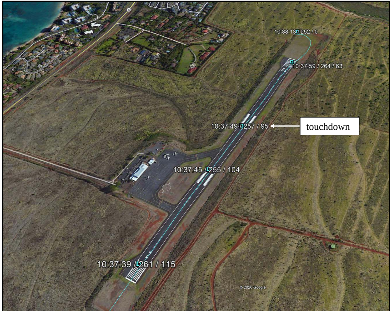
Figure 6: HJH with Time (HST) /Altitude (ft) / Indicated Airspeed (kt) Recorded on G1000 (Note: runway slopes up approximately 15 ft from runway 2 threshold to runway 20.)
